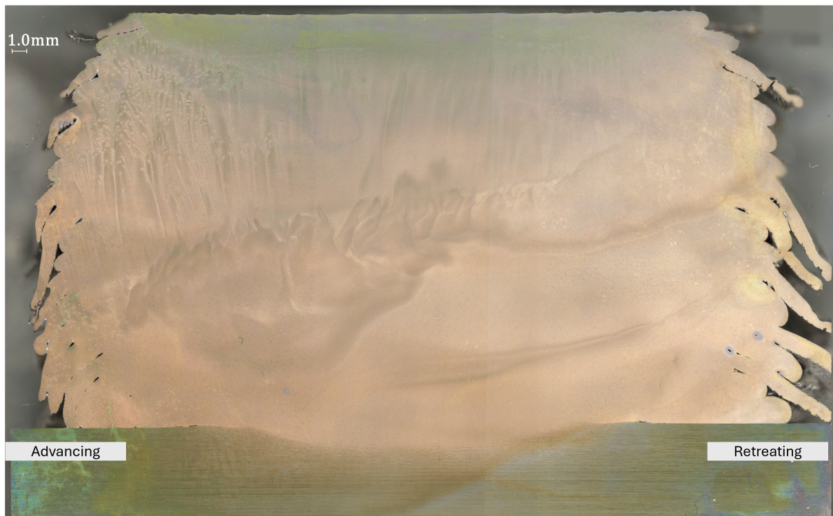
Figure 4.18: Optical micrograph taken of a no pause cross section on a Keyence VHX 7000x Optical Microscope.
