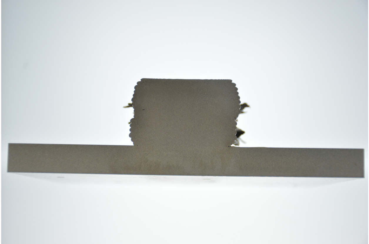
Figure A.8: Photo of sample 1a after cutting for contour measurement.
