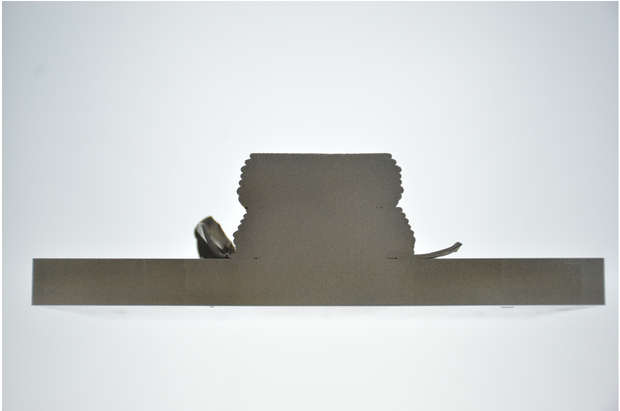
Figure A.21: Photo of sample 2a after cutting for contour measurement.
