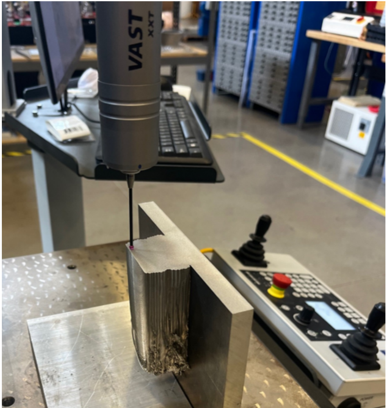
Figure 3.10: (a) Image of the ZEISS DuraMax CMM measuring a cut face of a sample for contour analysis.
