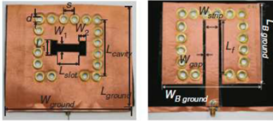
Figure 2.3: Substrate Integrated Waveguide Cavity-Backed Dog-Bone Slot Antenna after (6).
