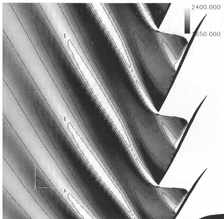
Figure 167. Details of Shock at Fan Blade Tips.
