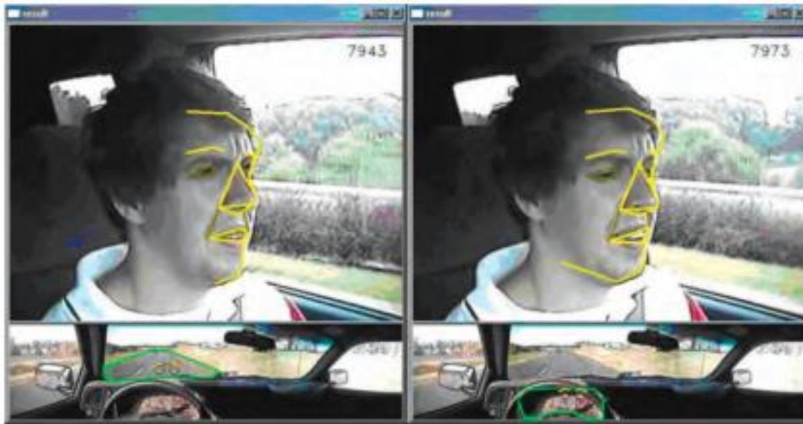
Figure 1. 6 Illustration of SHRP2-NDS Video: Capturing Driver Distraction and Gaze (Source: (Campbell 2012))
