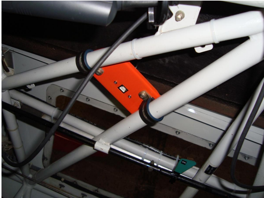
Figure 21: USB to Serial Hub connection for AHRS in Right-Side, Forward Cockpit
