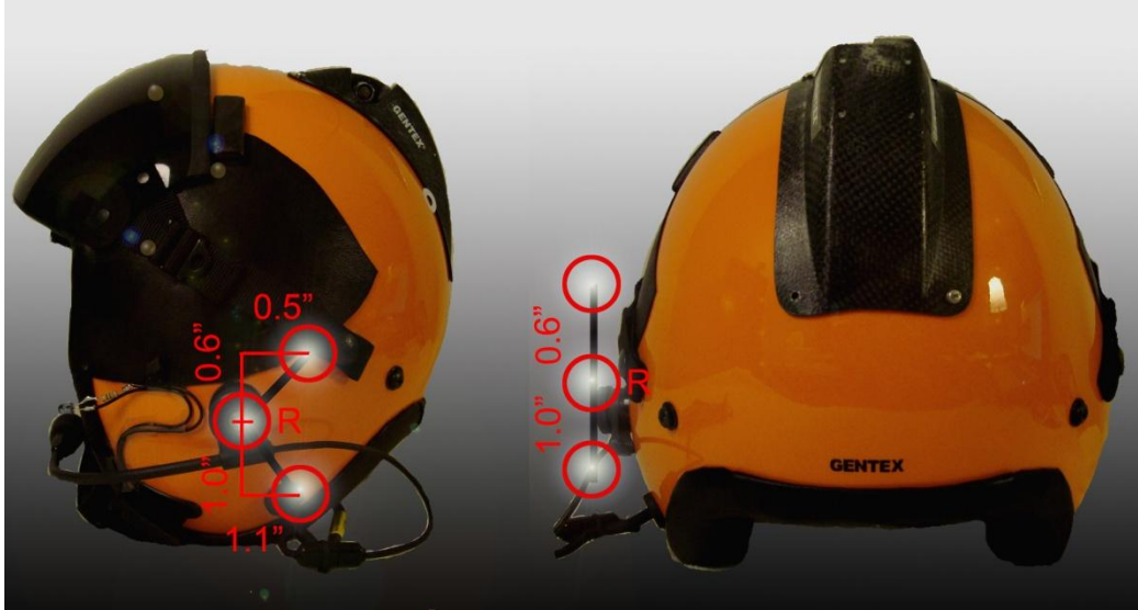
Figure 19: Final Installation of IR-LEDs for use in Aircraft Forward Seat
