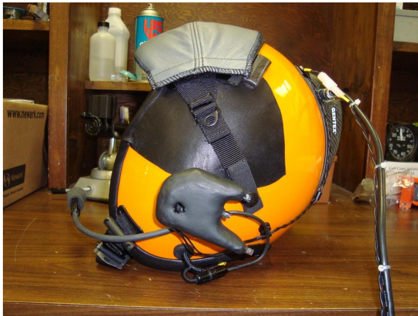
Figure 20: Upgraded Helmet with Custom Made IR-LED Mount
