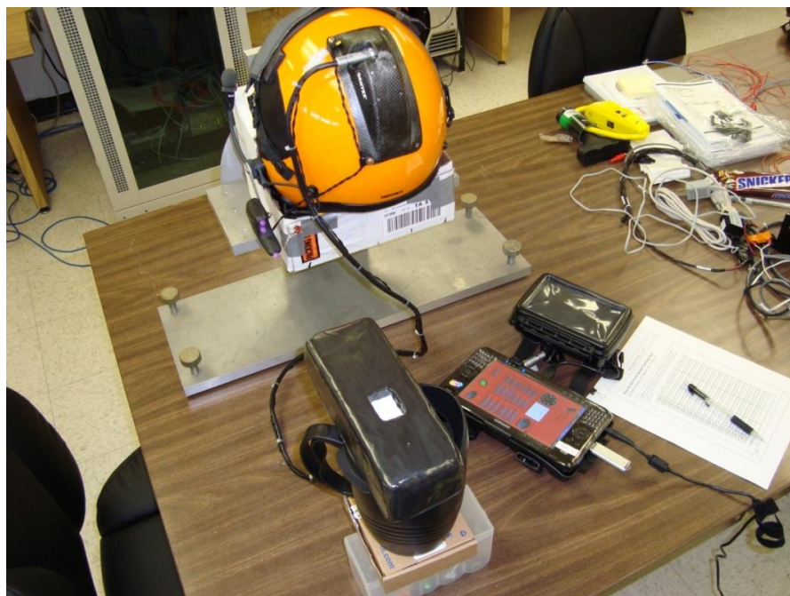
Figure 26: Calibrating IR Camera for Roll Angles
