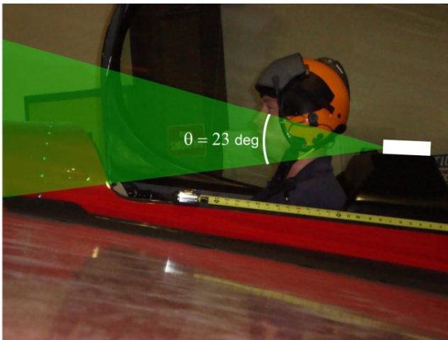
Figure 18: Proposed Locations of Camera in Relation to Forward and Rear Seats of Aircraft
