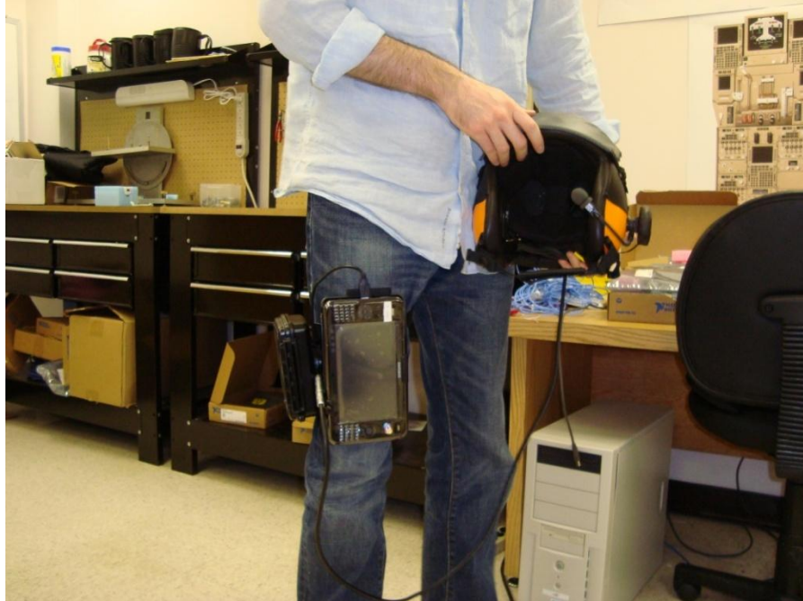
Figure 23: Demonstration of Leg-Mount System
