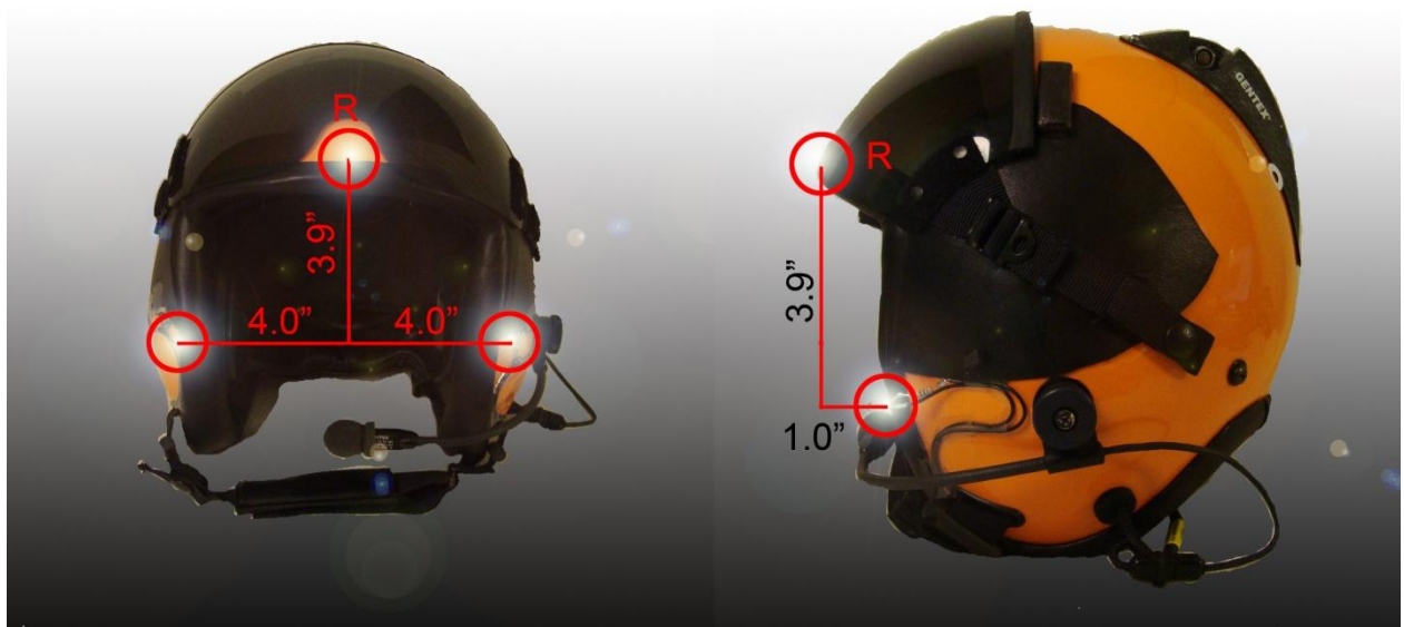
Figure 17: Initial Installation of Infrared LEDs for use in Rear Seat of Aircraft
