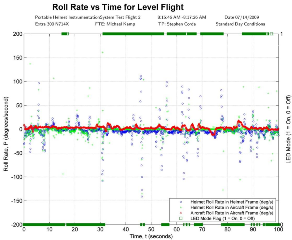
Figure 46: Roll Rate versus Time for Level Flight
