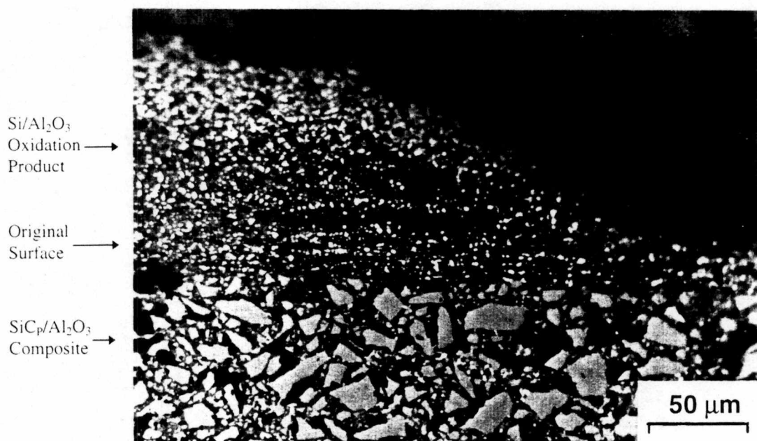
Figure 4-9. Optical microphotograph of cross-sectional view of the SiC p /Al 2 O 3 composite corroded at 1200°C for 150 hours after silicates removed with a HF solution showing Si/Al 2 O 3 oxidation product on surface.
