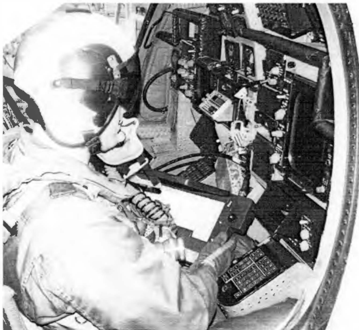
Figure 2: Panasonic CF-25 Laptop in EA-6B Prowler (Side View)
