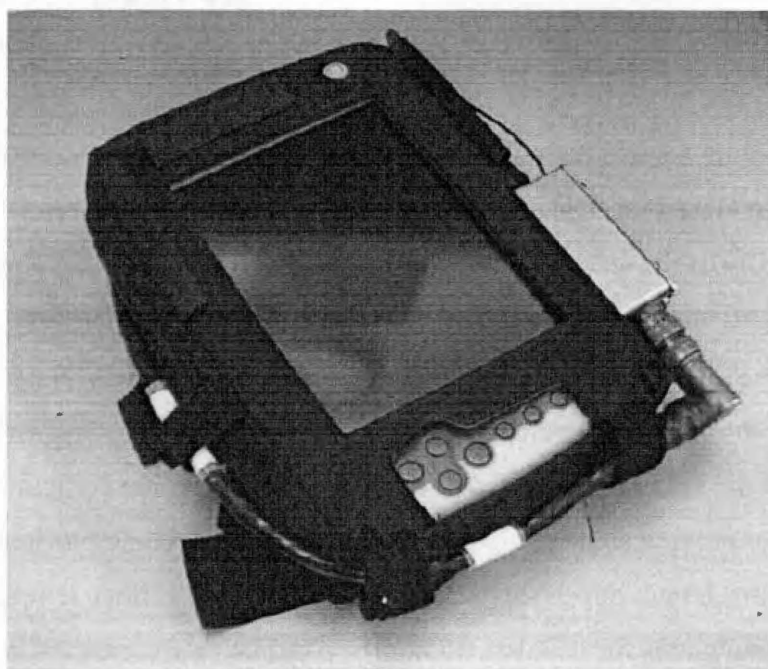
Figure 20: Velcro Strap for Panasonic Laptop for EA-6B
