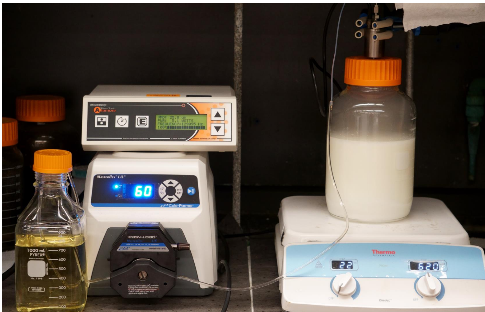
Figure 40 Alternative setup of the ultrasonic spraying to try and limit turbulence from overhead stirring by using magnetic stirring.
