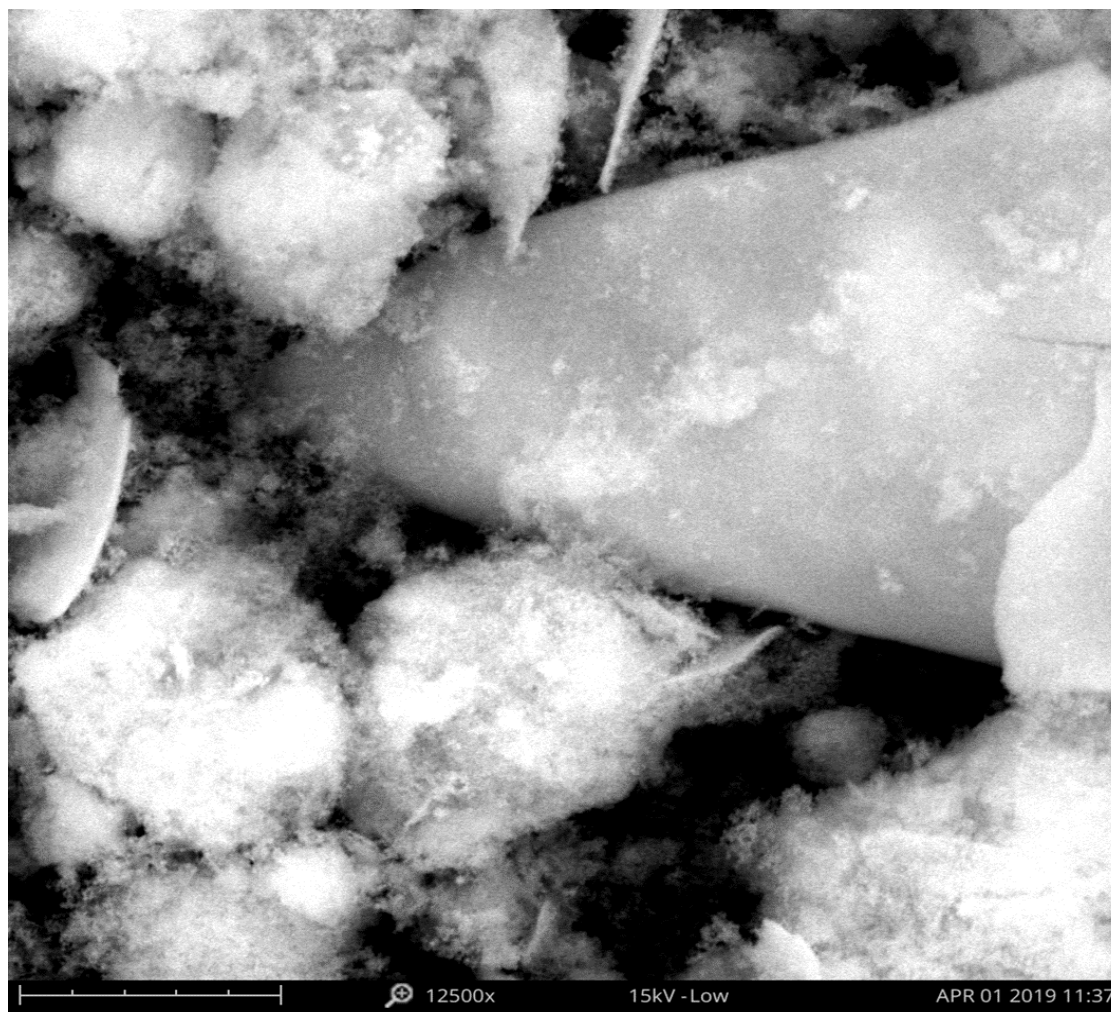
Figure 37 Powder resulting from the dripping of solution into the spray co-precipitated setup when a lid was put on to catch the ejected liquid.
