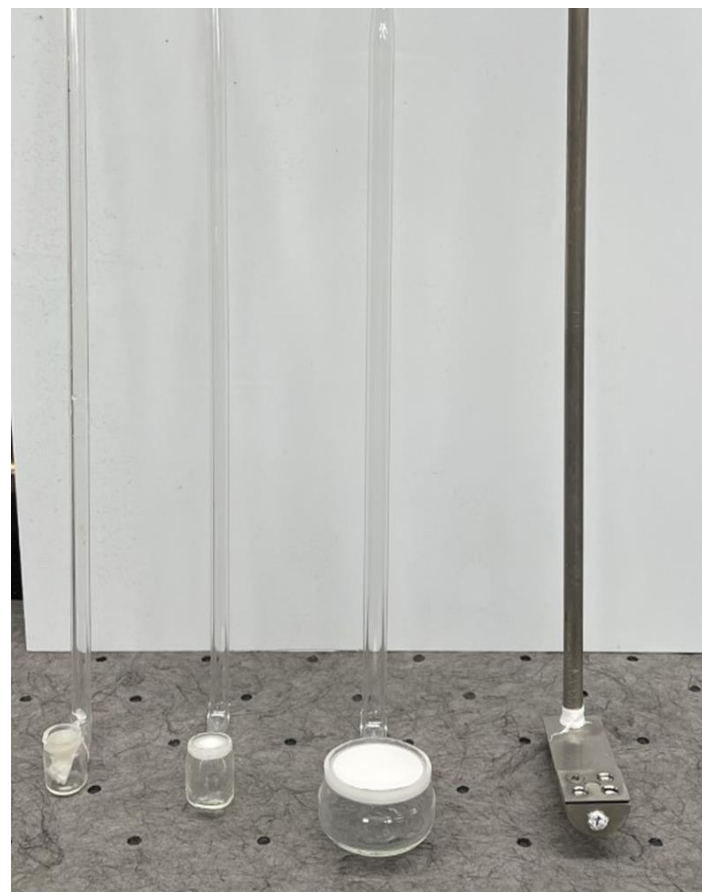
Figure 44 Side profile (left) and front profile (right) of the evolution of frits designed and improved for these studies.
