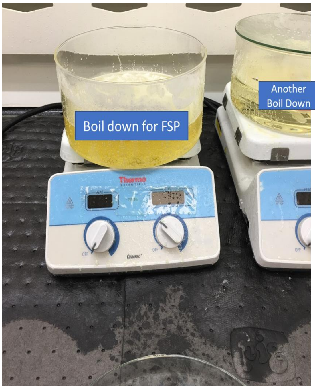
Figure 18 An example of a boil over if the solution was not fully cooled and alcohol was added. The darker yellow color is attributed to dissolved NO x .
