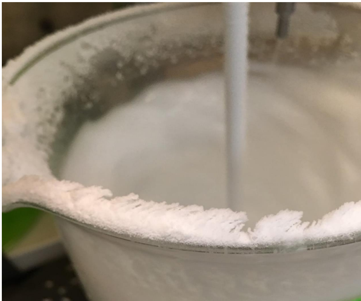
Figure 39 Precipitated spray powder collecting on the lip of the beaker from the turbulent air ejecting the ultrasonic spray.
