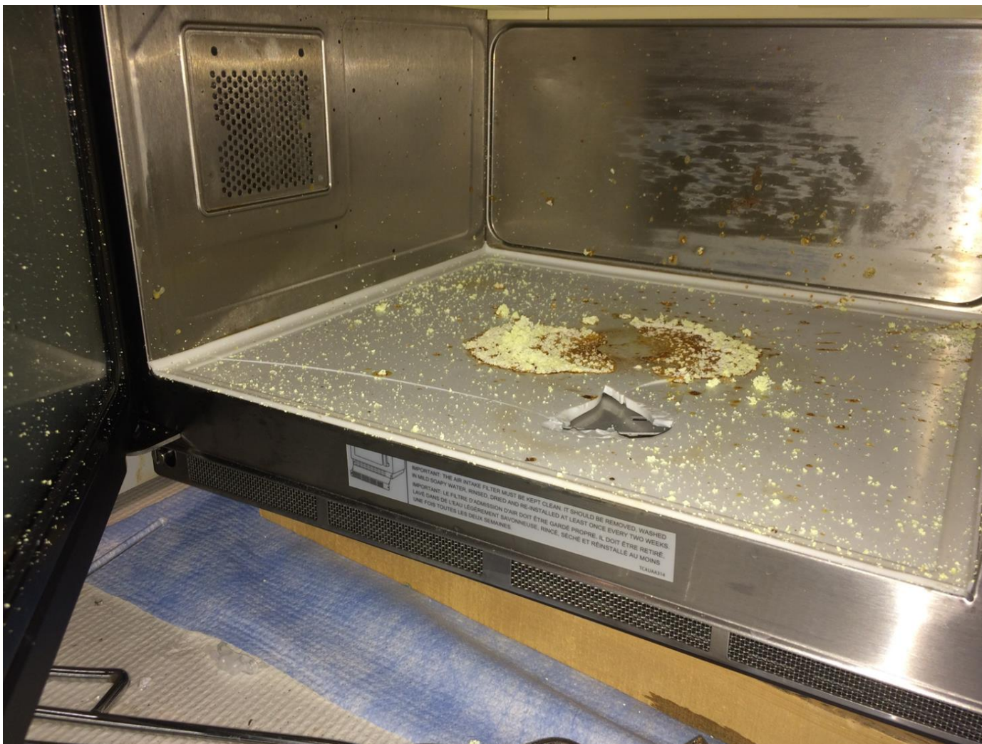
Figure 16 Example of the corrosion and wear from repeated use in microwave assisted solution combustion synthesis experiments.
