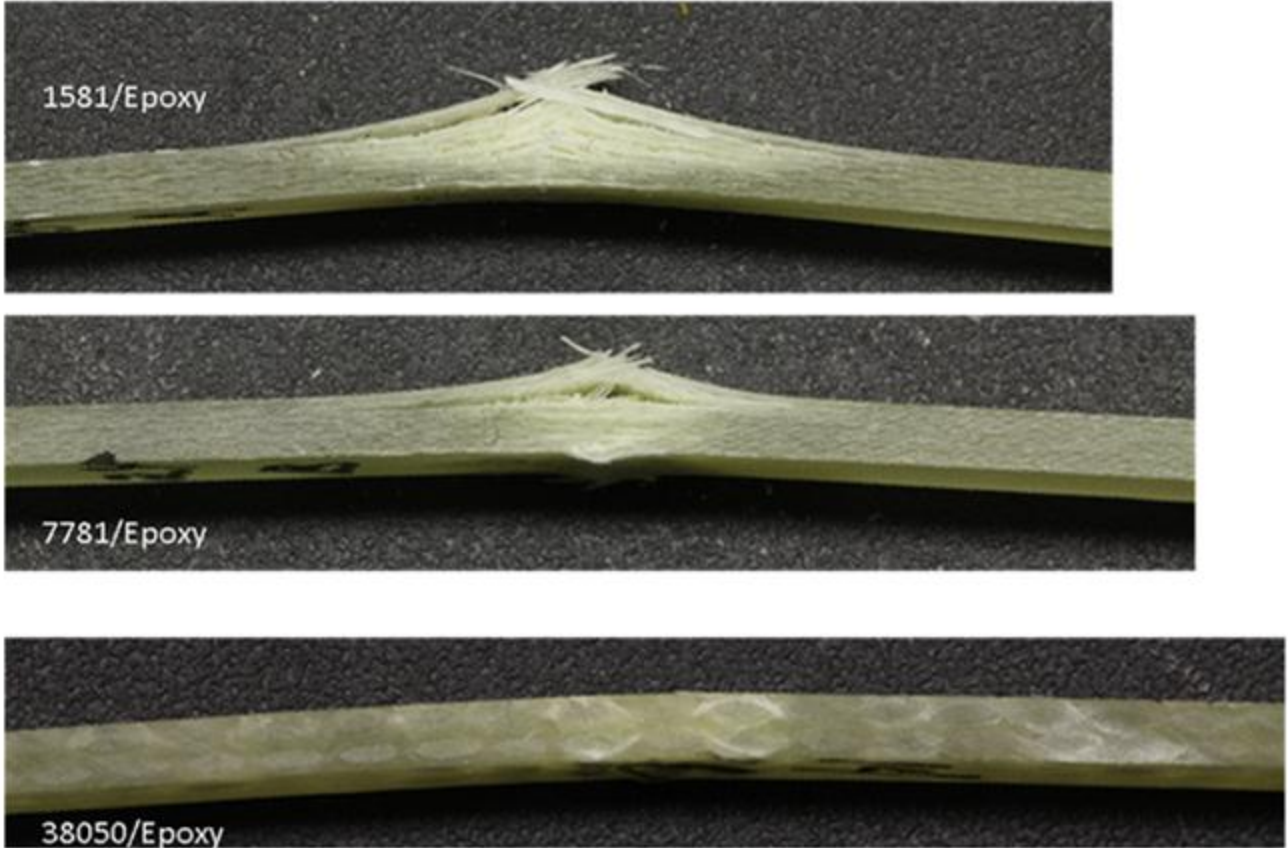
Figure 32. Photographs of the side view of the failed samples' middle sections tested at 77K showing the failure pattern.
