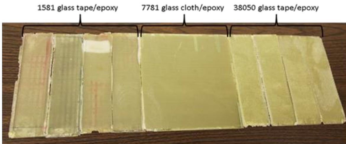
Figure 20. The three types of composite plates fabricated using the VPI process.
