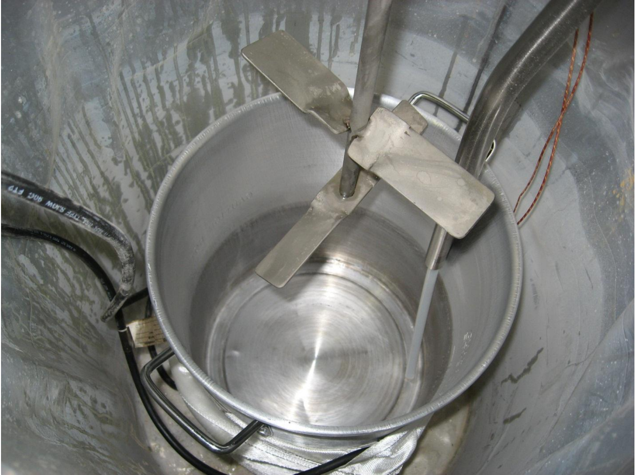
Figure 17. Inner container where mixing of resin occurred.
