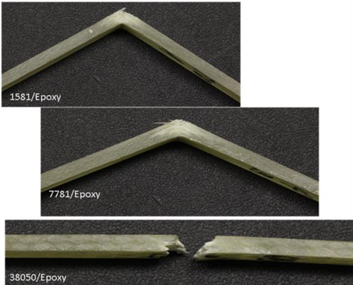
Figure 31. Photographs of the side view of the failed samples' middle sections tested at 295K showing the failure pattern.
