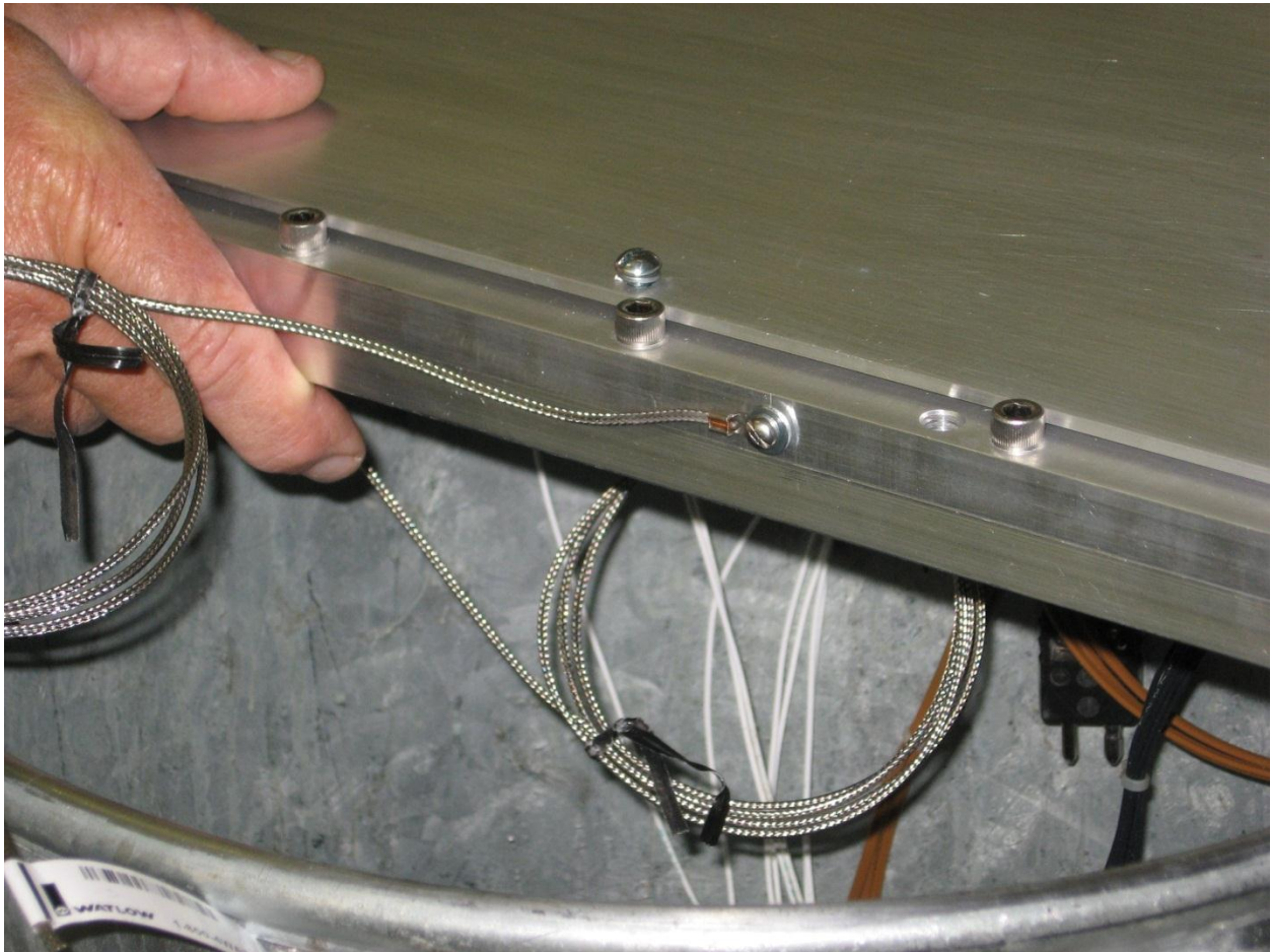
Figure 14. Thermocouple connected to side of mold plate.
