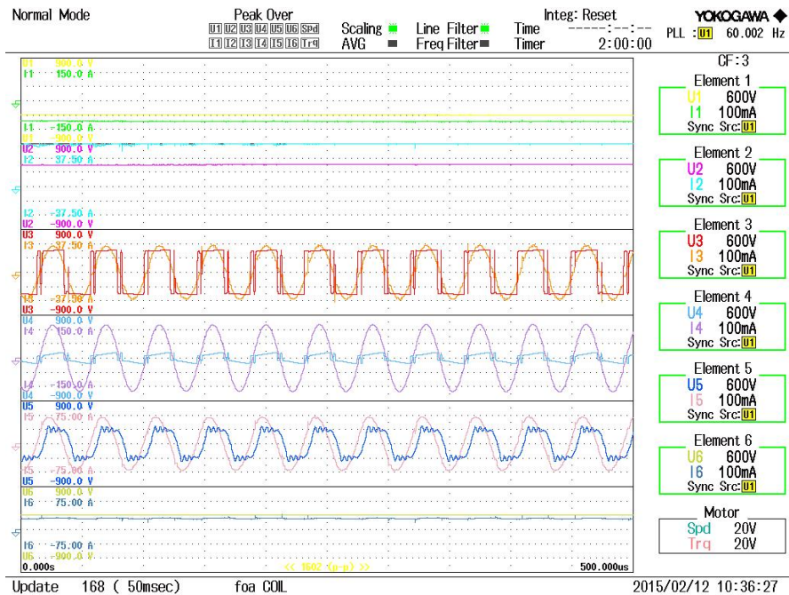
Figure 5-27. The inverter, transformer, coil, and rectifier output waveforms.
