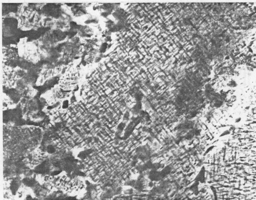
Figure 48. Al-8 wt% Fe aged at 300 °C for 100 hours, TEM, 62,000X. Complete transformation to oriented needles of Al 3 Fe, θ', in the grains. The grain boundary phase is still Al 6 Fe.
