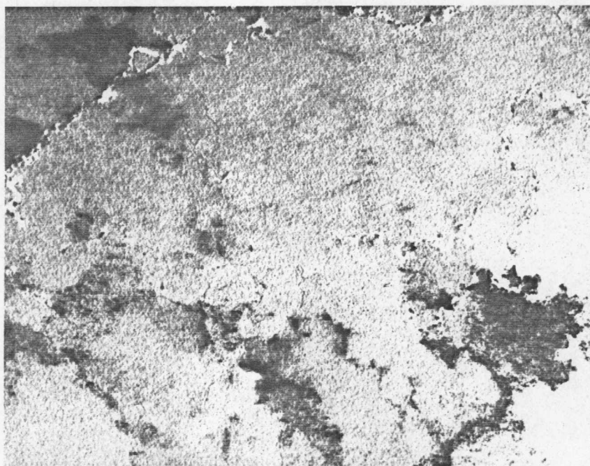
Figure 50. Al-8 wt% Fe-3.4 wt% Ce aged at 300 °C for 1 hour, TEM, 62,000X. Formation of fine spheroidal zones, \theta'' , in the grain. Fine precipitation at the grain boundary.
