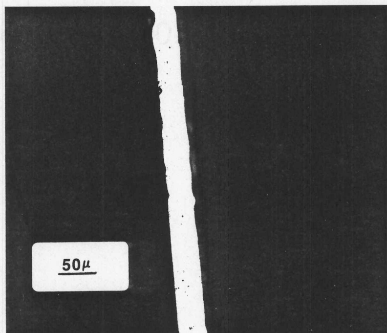
Figure 27. Al-8 wt% Fe-3.4 wt% Ce, as quenched, Keller's etch, 200X. Complete Zone A, no second phase reflections present as shown in the diffractometer scan above.
