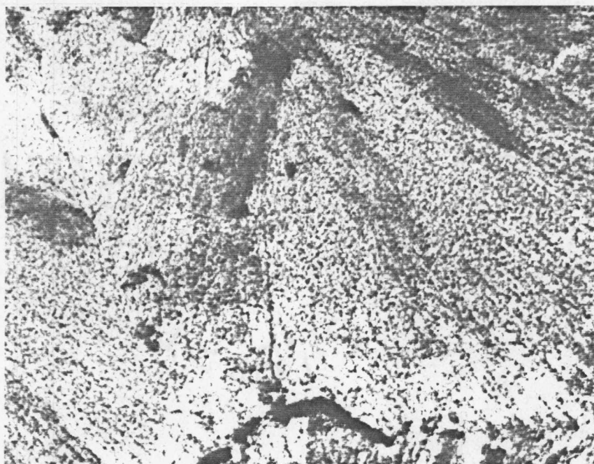
Figure 50. Al-8 wt% Fe-3.4 wt% Ce aged at 300 °C for 1 hour, TEM, 62,000X. Formation of fine spheroidal zones, \theta'' , in the grain. Fine precipitation at the grain boundary.
