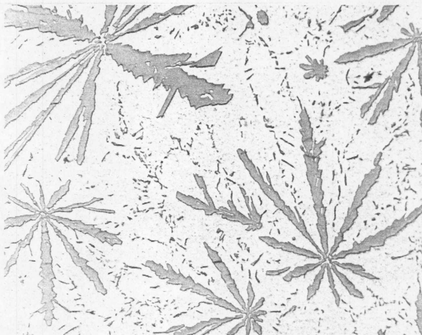
Figure 21. Al-8 wt% Fe, cast master alloy, HF etch, 680X. Figure shows coarse, irregular \alpha -Al-Al 3 Fe eutectic.
