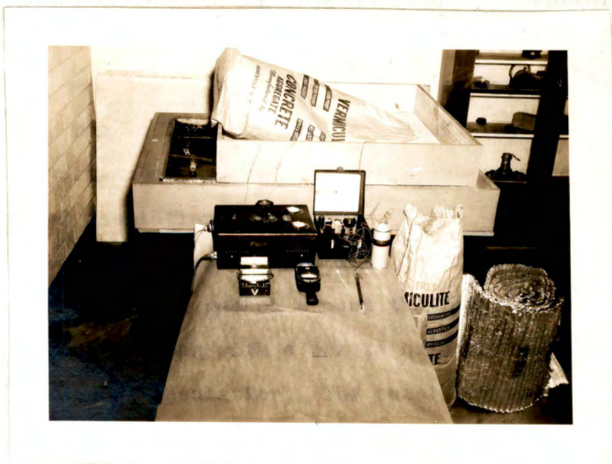
Fig. No. 6 View of Laboratory Calorimeter Showing Wattmeter, Cutter, Voltmeter, and Insulation.
