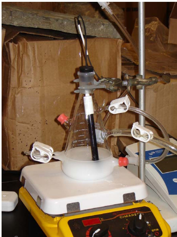
Figure 5. Experimental vessel with immersed pH electrode allowed for reactant input and aliquot withdrawal without exposure to the ambient atmosphere.
