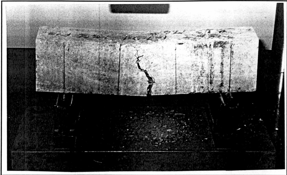
SFRC BEAM AT FAILURE HAVING 3/4-INCH FIBERS AT 1.5% VOLUME.
