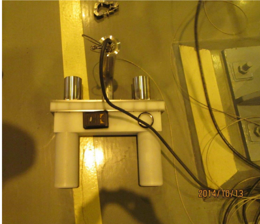
Figure 5. A fork detector used to verify spent nuclear fuel [12].
