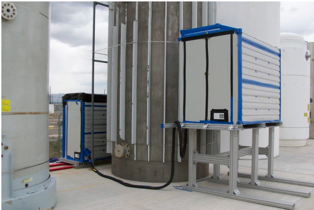
Figure 8. Image of two planar drift tube detectors for muon tomography surrounding a spent fuel cask [16].
