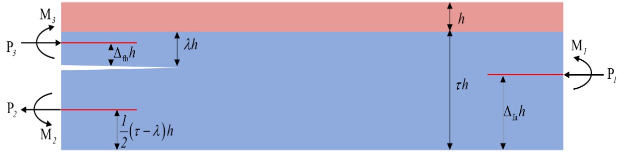
Figure 2.4. The model of film/substrate system with crack
