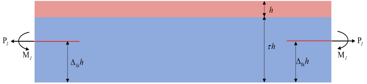
Figure 2.3. The model of film/substrate system without crack
