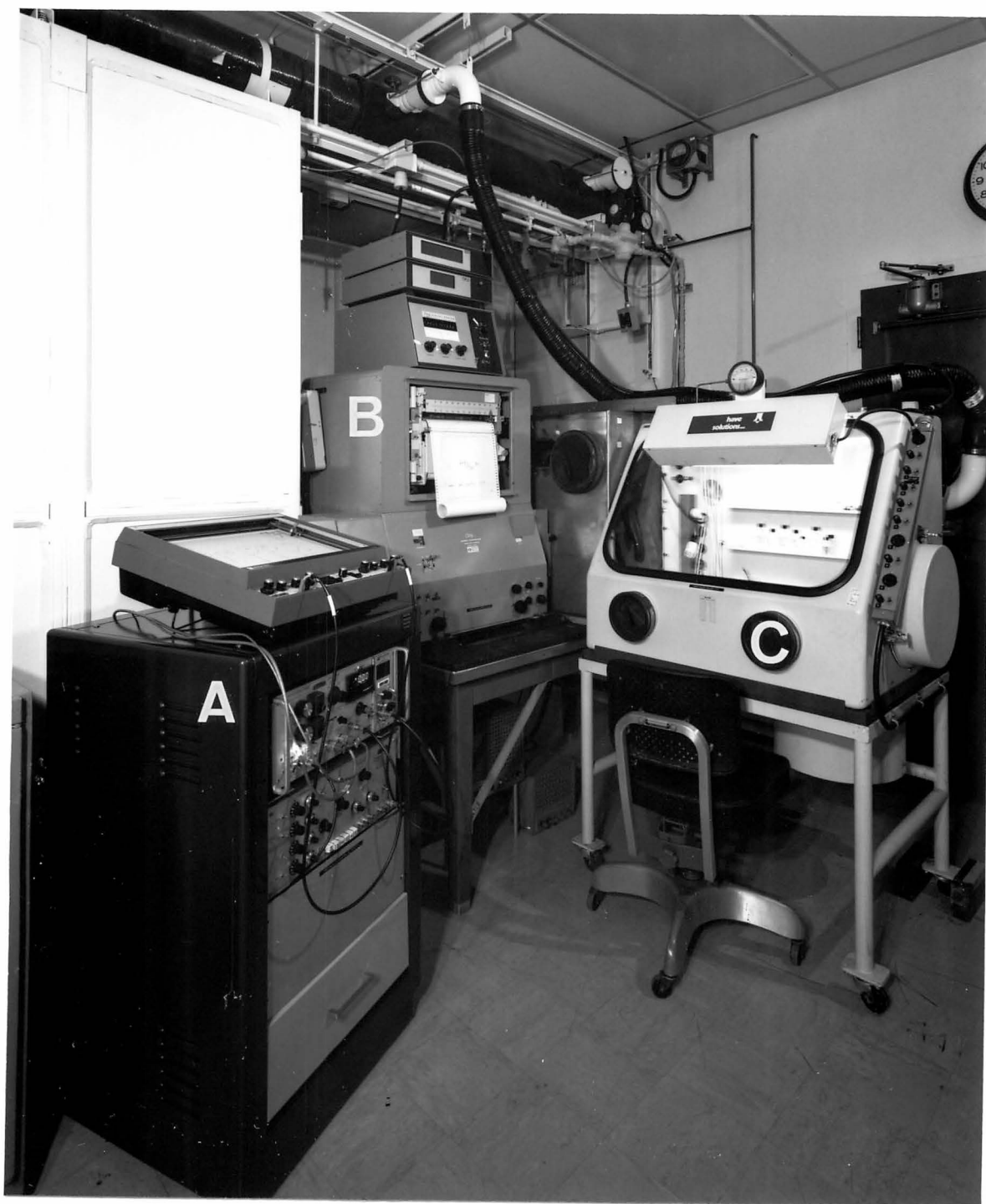
Figure 3. Equipment for spectroelectrochemical studies of radioactive actinide elements. Voltammeter (A), spectrophotometer (B), and modified glove box (C).
