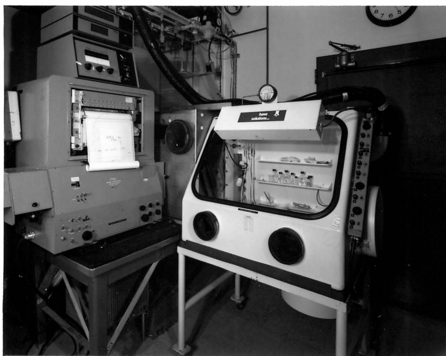
Figure 4. Spectrophotometer/modified gloved box assembly. Gloved box removed from spectrophotometer (upper photo) and installed in spectrophotometer (lower photo).
