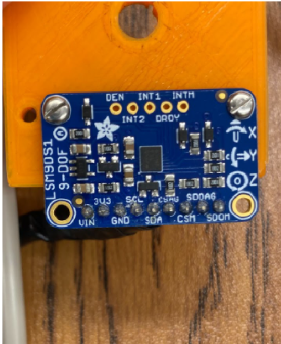
Figure A.3: Picture of the IMU fixed onto its mounting plate
