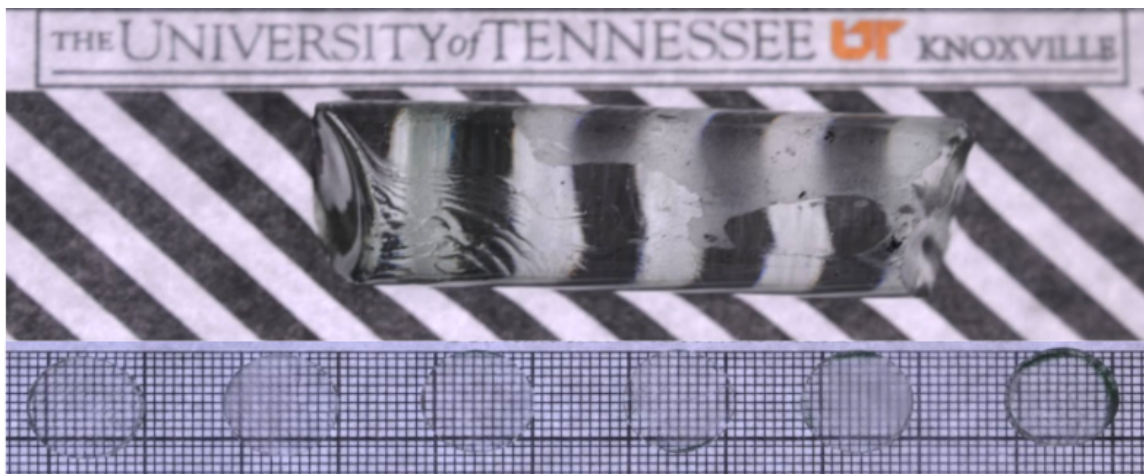
Figure 3.26: CsI:Na,Sm(0.3,0.01)% Crystal qualities. Top left: crystal after extraction from ampoule. Bottom: Slabs cut from the main boule in ascending order from left to right. Top right: Image of slice 6, the slice with the most visible inclusions and impurities.
