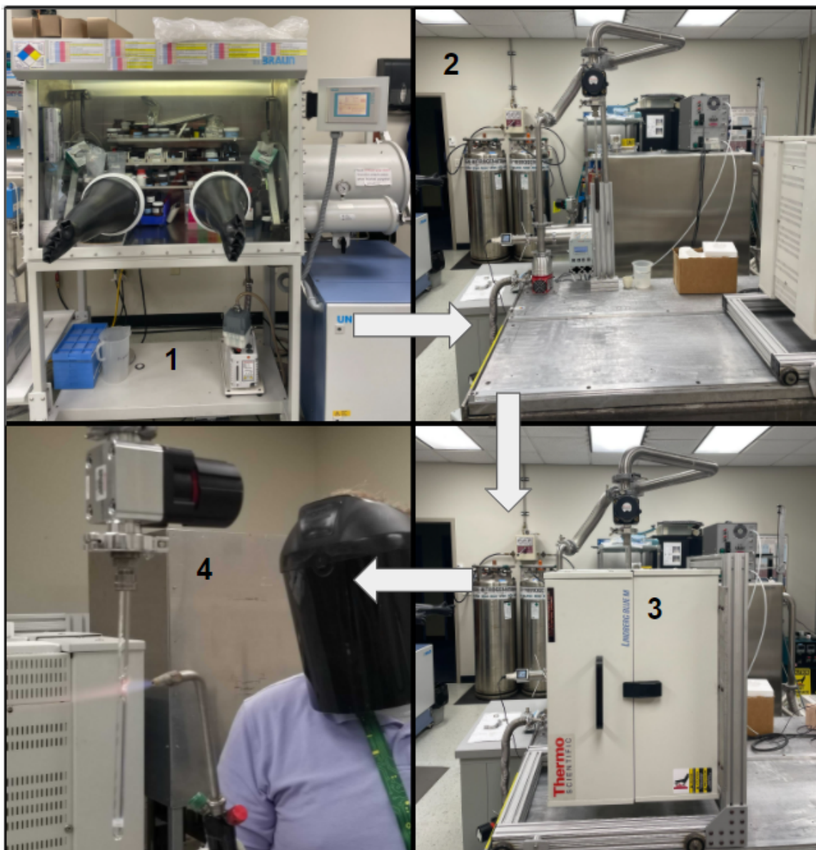
Figure 2.3: [1]: ampoule loading glovebox. [2]: Ampoule on vacuum station. [3]: Ampoule being baked out under vacuum. [4]: Ampoule being sealed with a hydrogen oxygen torch.
