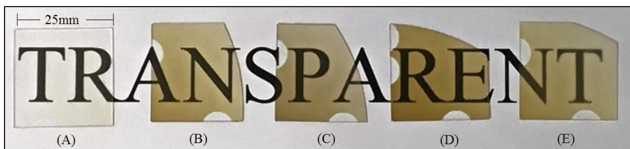
Figure A2. ZLANI glass films deposited by PLD for (A) 30 min, (B) 1 hour, (C) 2 hours, (D) 3 hours, (E) 4 hours). The witness marks where the substrates were mounted to the substrate holder can be seen in images B-E.
