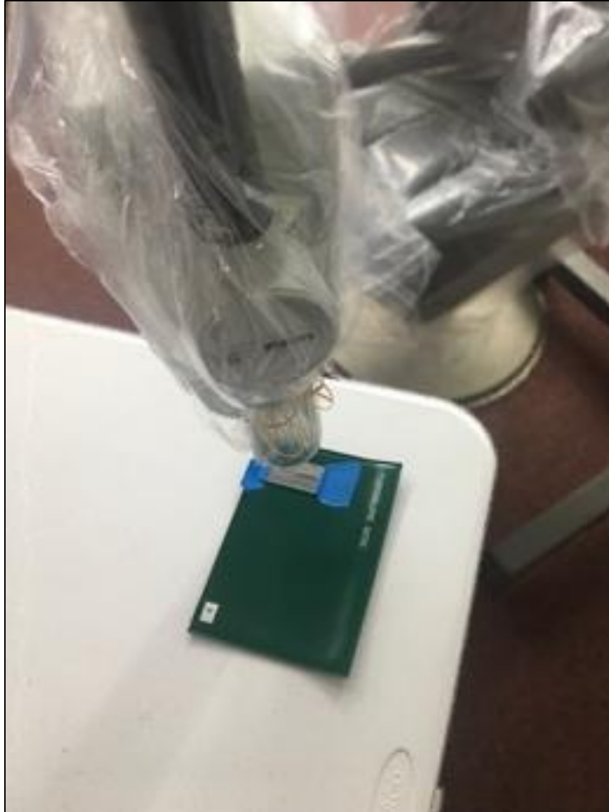
Figure 25. X-ray tube utilized for reported experiments. It is shown here directed at image phantom overlaying a medical imaging plate within a light tight envelope.
