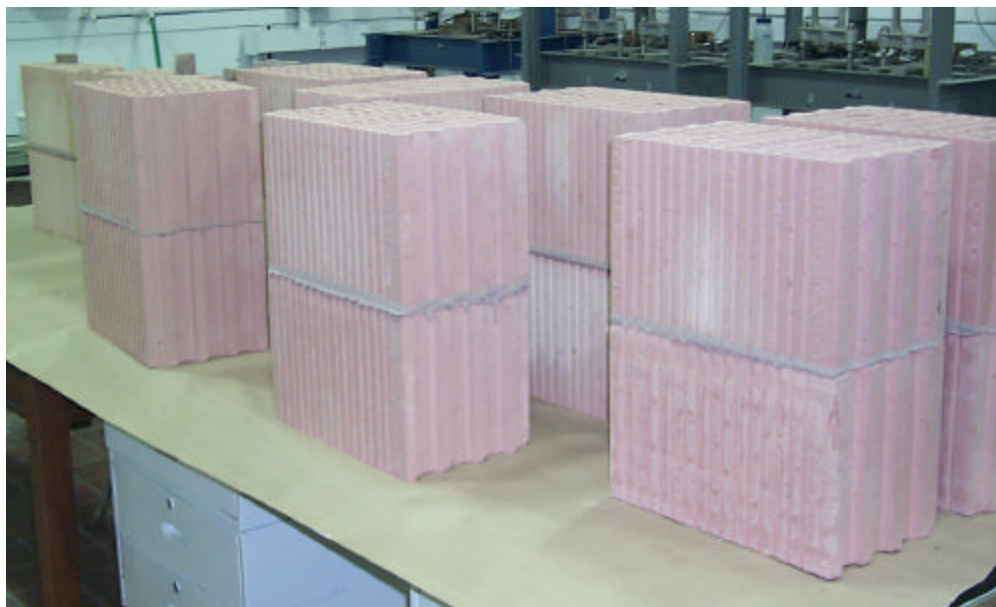
FIGURE 3.4 - Prisms 3-4 Days After Construction
