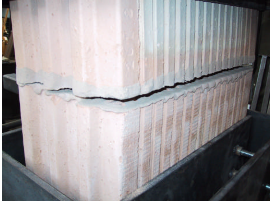
FIGURE 3.13 - Prism After Flexural Failure
