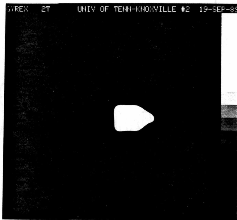
Figure 54. Pseudo-3D ^{11}\text{B} MR image of a 0.5 M \text{NaBPh}_4 phantom using the single point reconstruction method.
