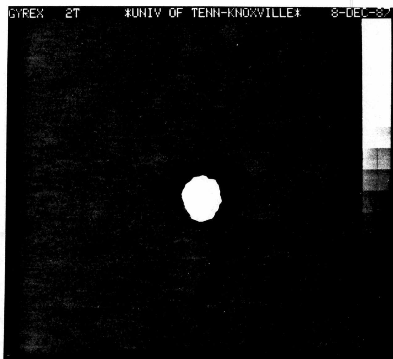
Figure 40. ^{11}\text{B} MR image of a 0.2 M \text{NaBPh}_4 phantom obtained using a three-dimensional gradient echo protocol.
