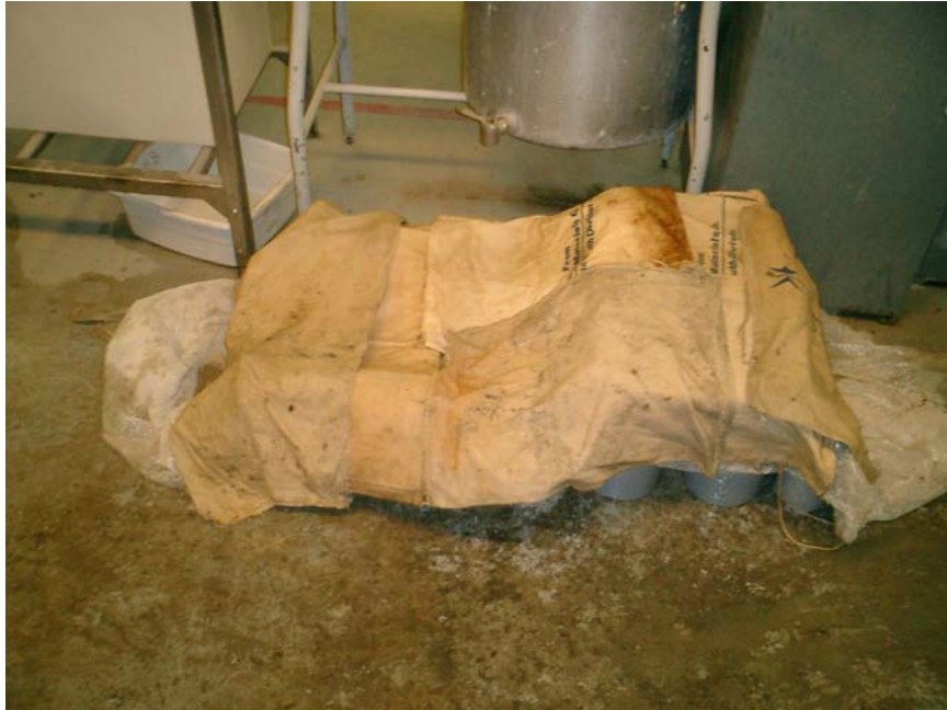
Figure B-6 Specimens After Casting
