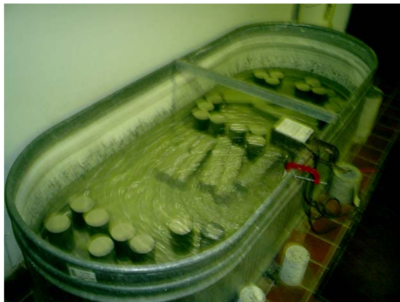
Figure B-7 Lime Water Bath
