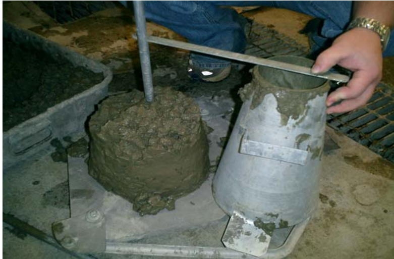
Figure B-8 Slump Test in Progress
