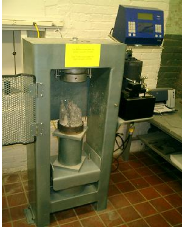
Figure B-10 Compressive Strength Machine After Test
