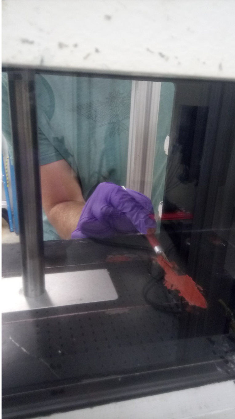
Figure 3.3: Photograph of wind tunnel test section with floor insert and mounted cylinder. Flow would be right to left. Vacuum grease is applied to the gap created by the floor insert. Excess grease is removed with an exacto knife.
