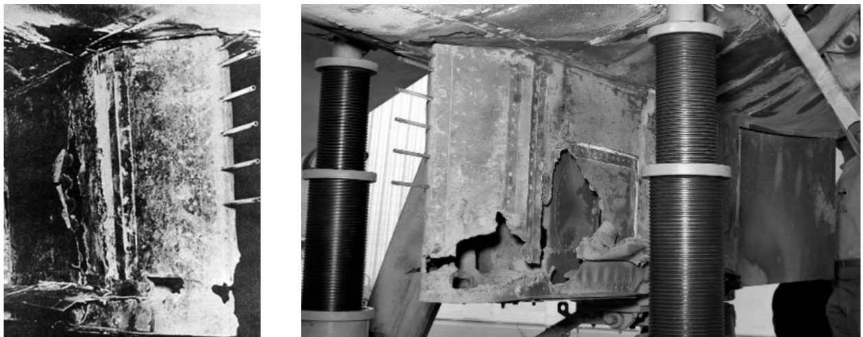
Figure 1.3: Pylon on the North American X-15 after Flight 188. The pylon carrying a dummy ramjet engine is severely damaged. Figure from Jones and Berry [11].
