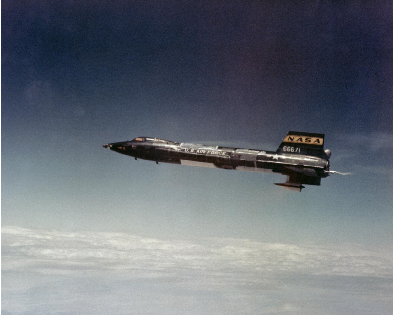
Figure 1.2: North American X-15 during a flight test. A dummy ramjet engine is carried on the underside of the vertical tail. Figure from NASA [9].
