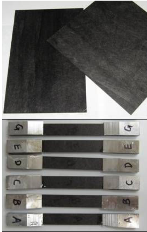
Figure 2.6 Specimen Preparation and Tensile Test Setup
