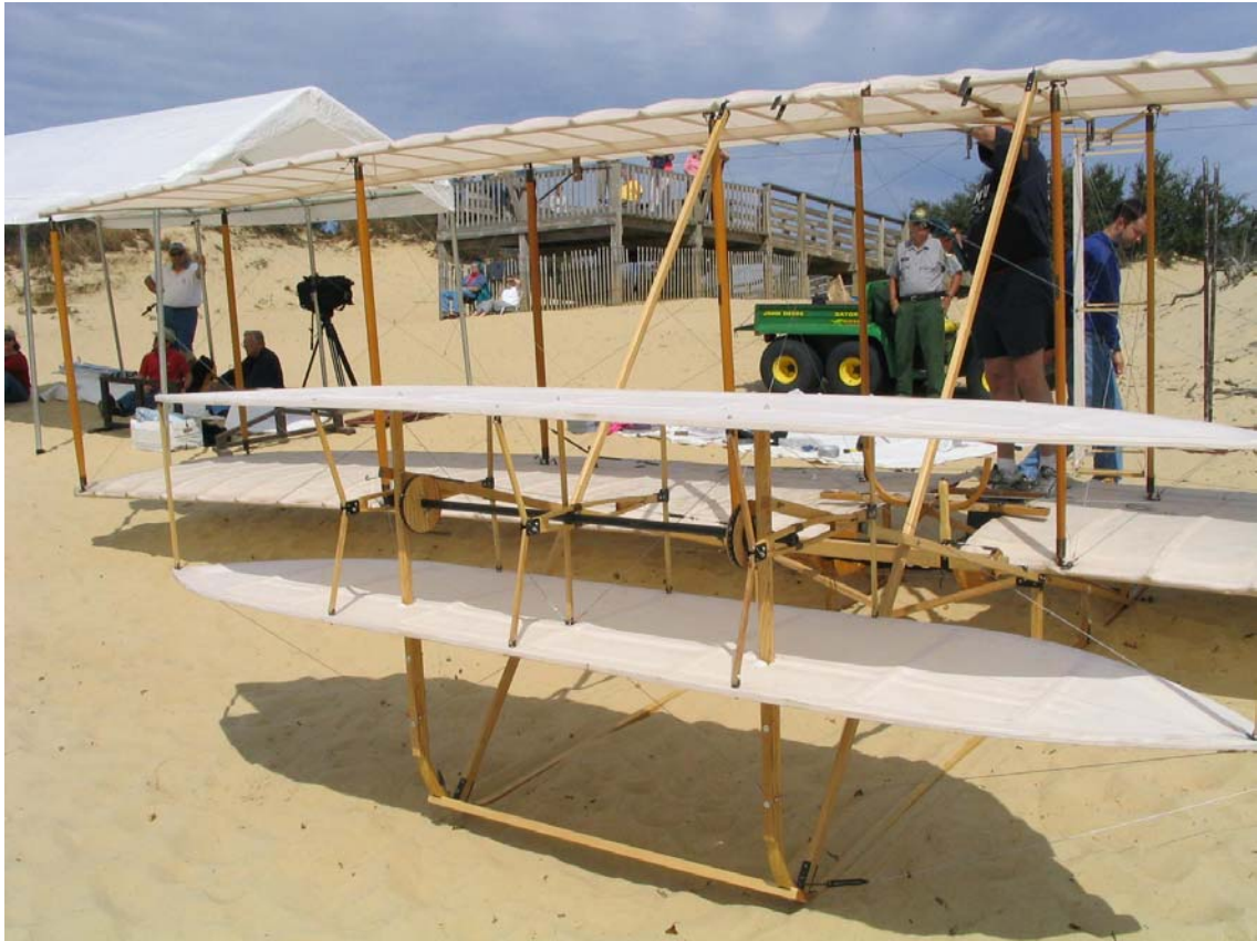
Figure B-1 Wright 1902.5 Canard Control System
