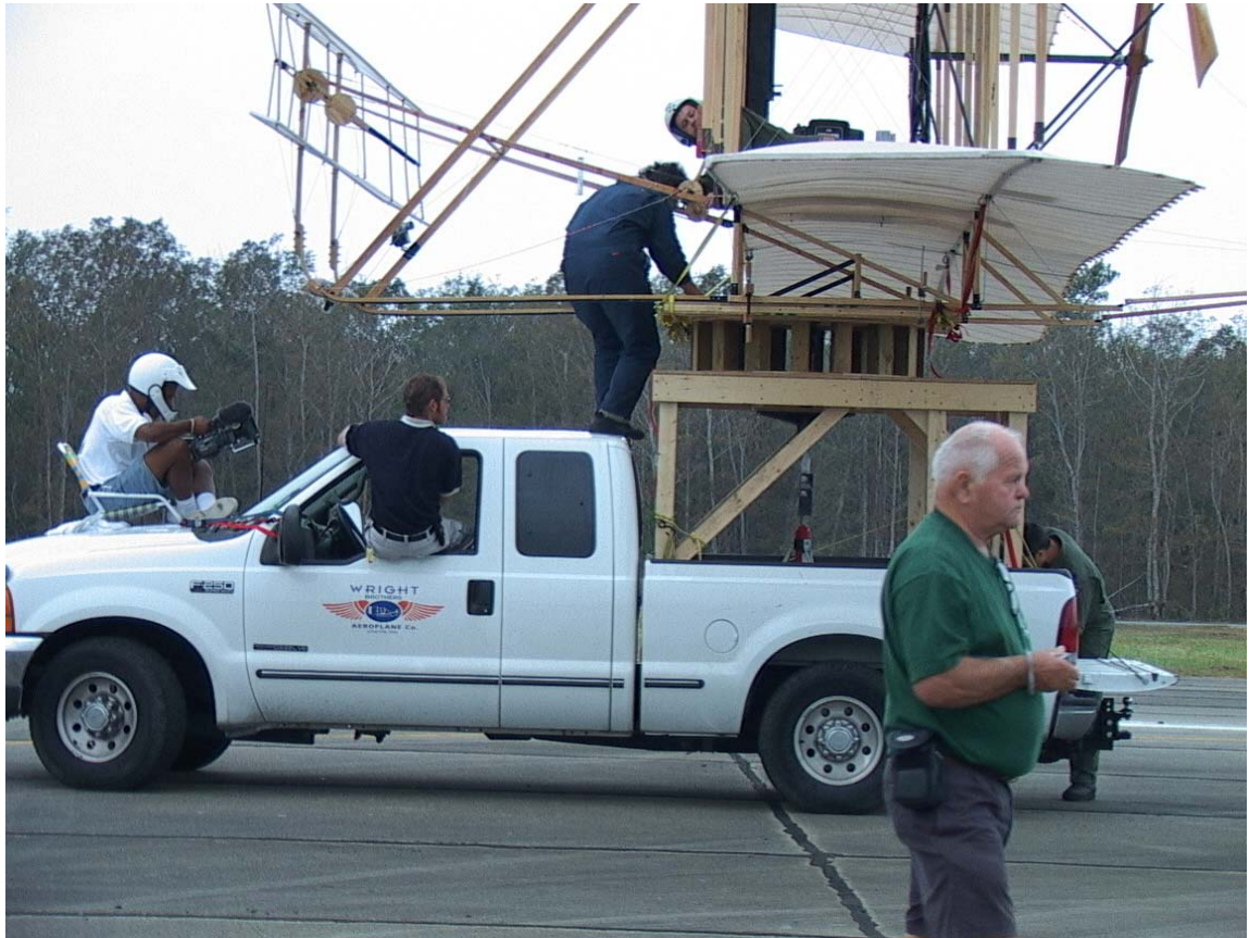
Figure 16 Wright 1903 Replica Mounted Atop Gimbal
