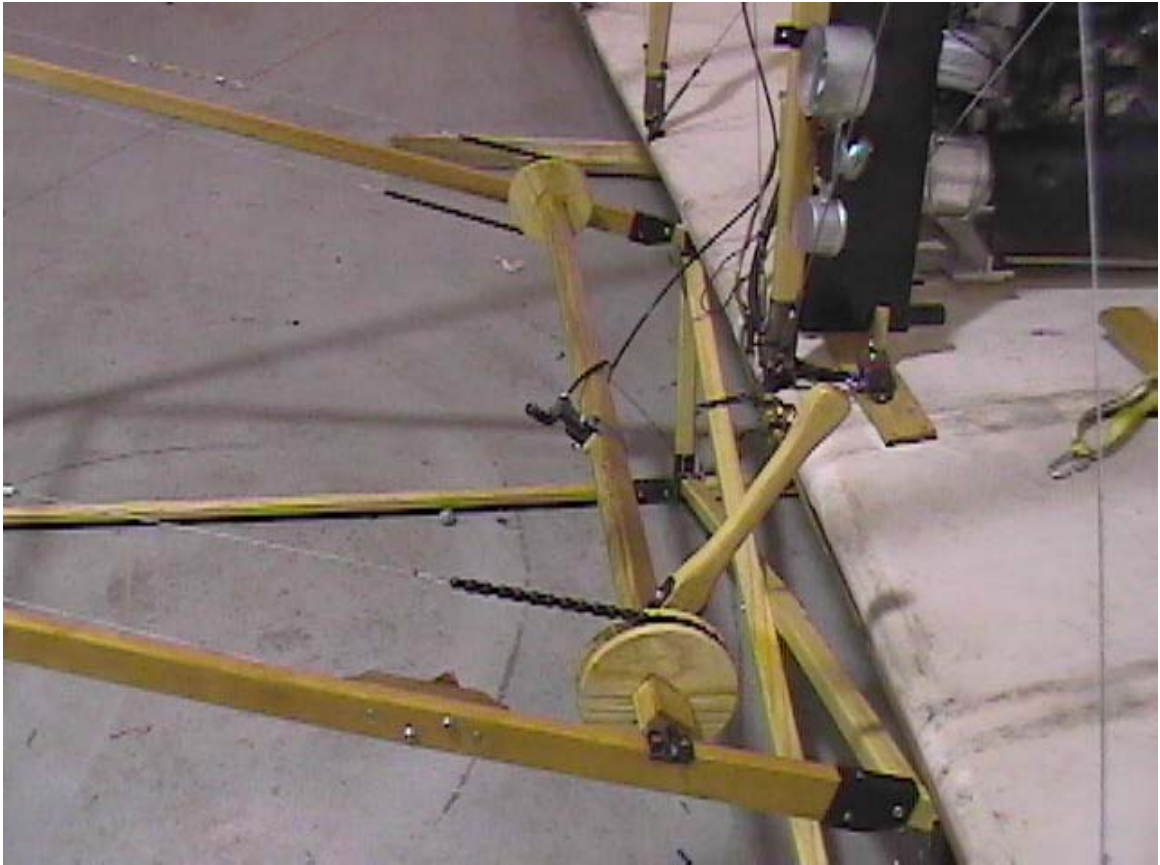
Figure 14 Wright 1903 Replica Pitch Control / Throttle Detail
