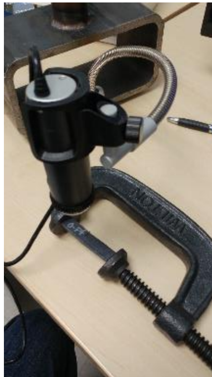
Figure 51 - Optical microscope setup
