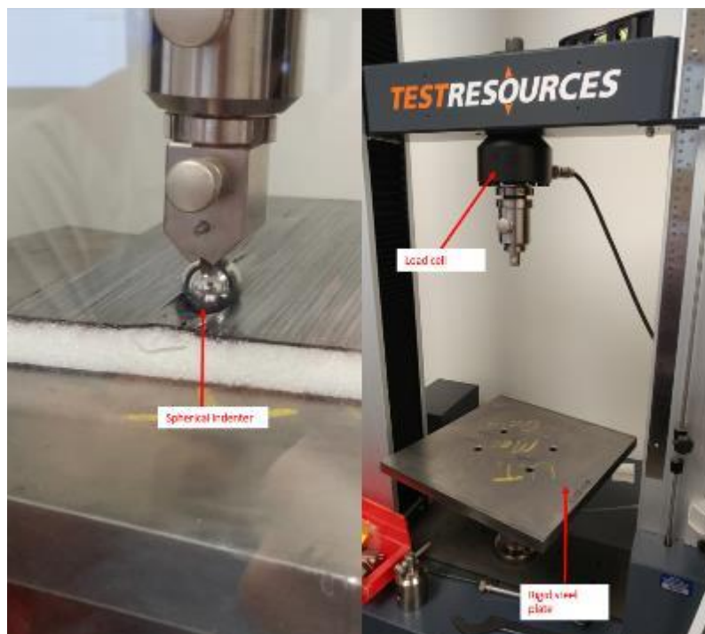
Figure 97 - Static indentation test setup for room temperature
