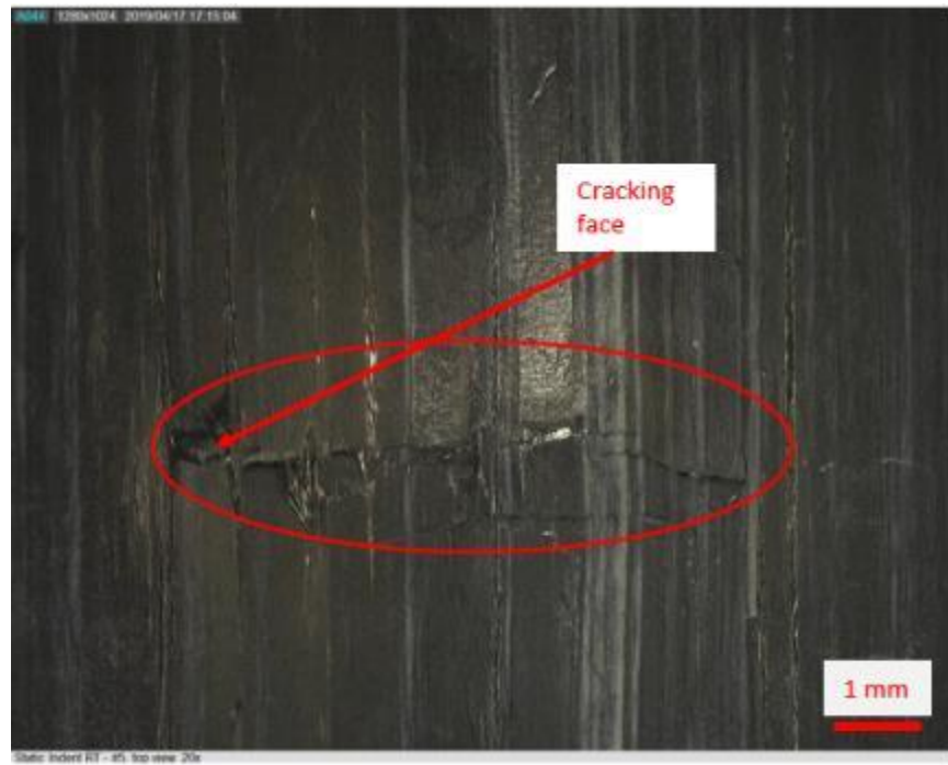
Figure 102 - Microscopy of RT static indent sample #5, top view of indent, 20x
