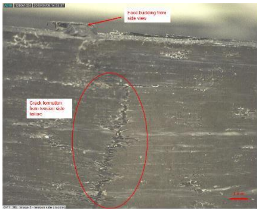
Figure 72 - Microscopy of 0-F1 flexural failure bottom view (tension side)
