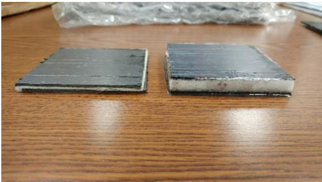
Figure 90 - PET film trial (left) vs huntsman epoxy (right)
