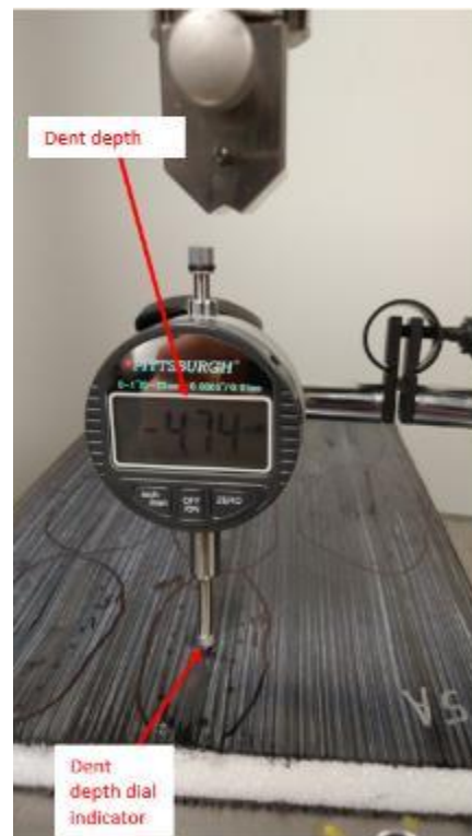
Figure 99 - Dent depth measurement process using dial indicator
