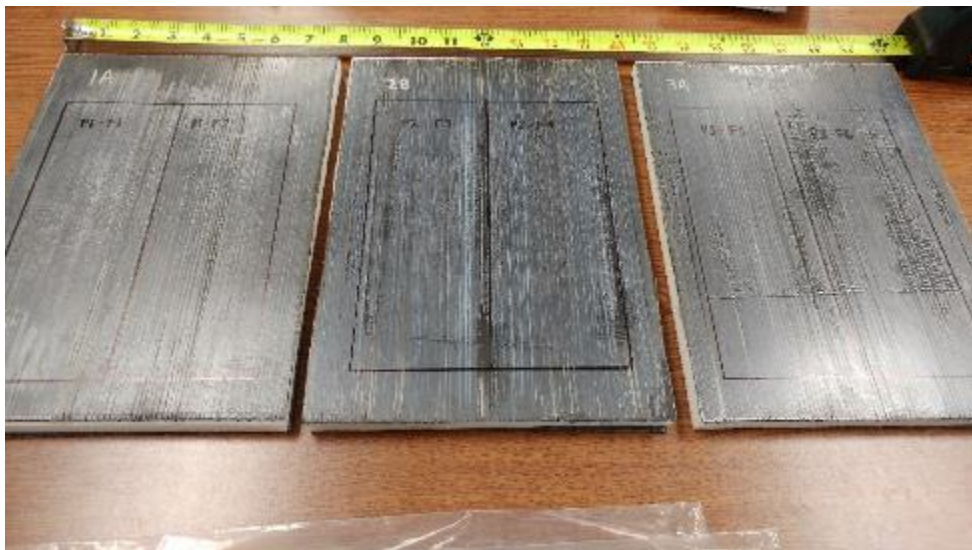
Figure 46 - Samples to be cut from sandwich panels
