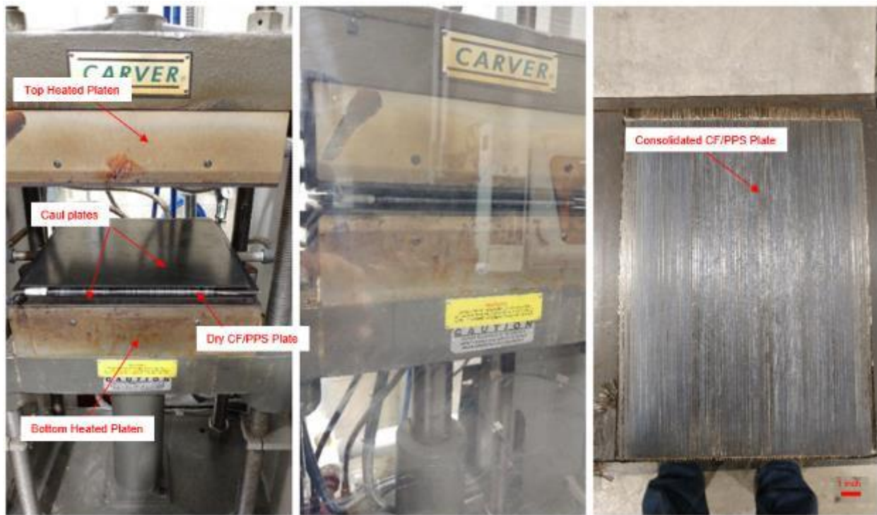
Figure 41 - Consolidation of CF-PPS through carver hot press
