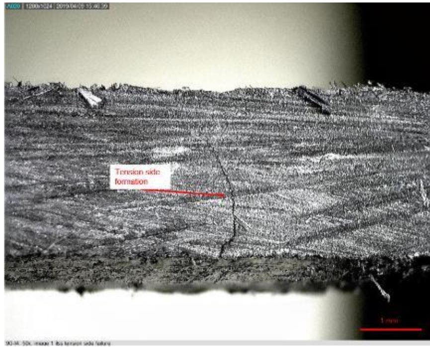
Figure 78 - Microscopy of 90-I4 ILSS failure side view
