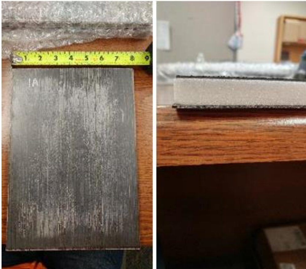
Figure 44 - Finished sandwich after bonding
