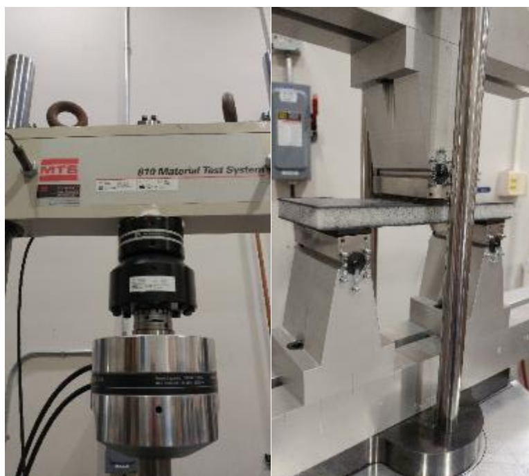
Figure 48 - Core shear testing setup
