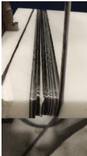
Figure 85 - Local crushing of foam during filament winding
