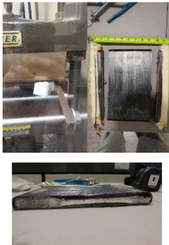
Figure 87 - Foam degradation during compression trial
