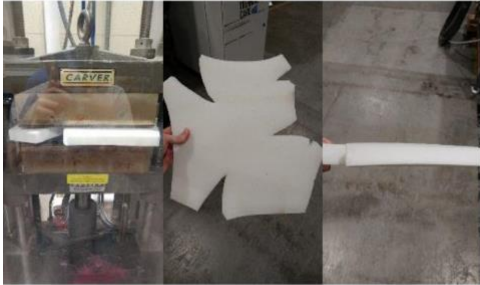
Figure 84 - Foam expansion during hot compression trial
