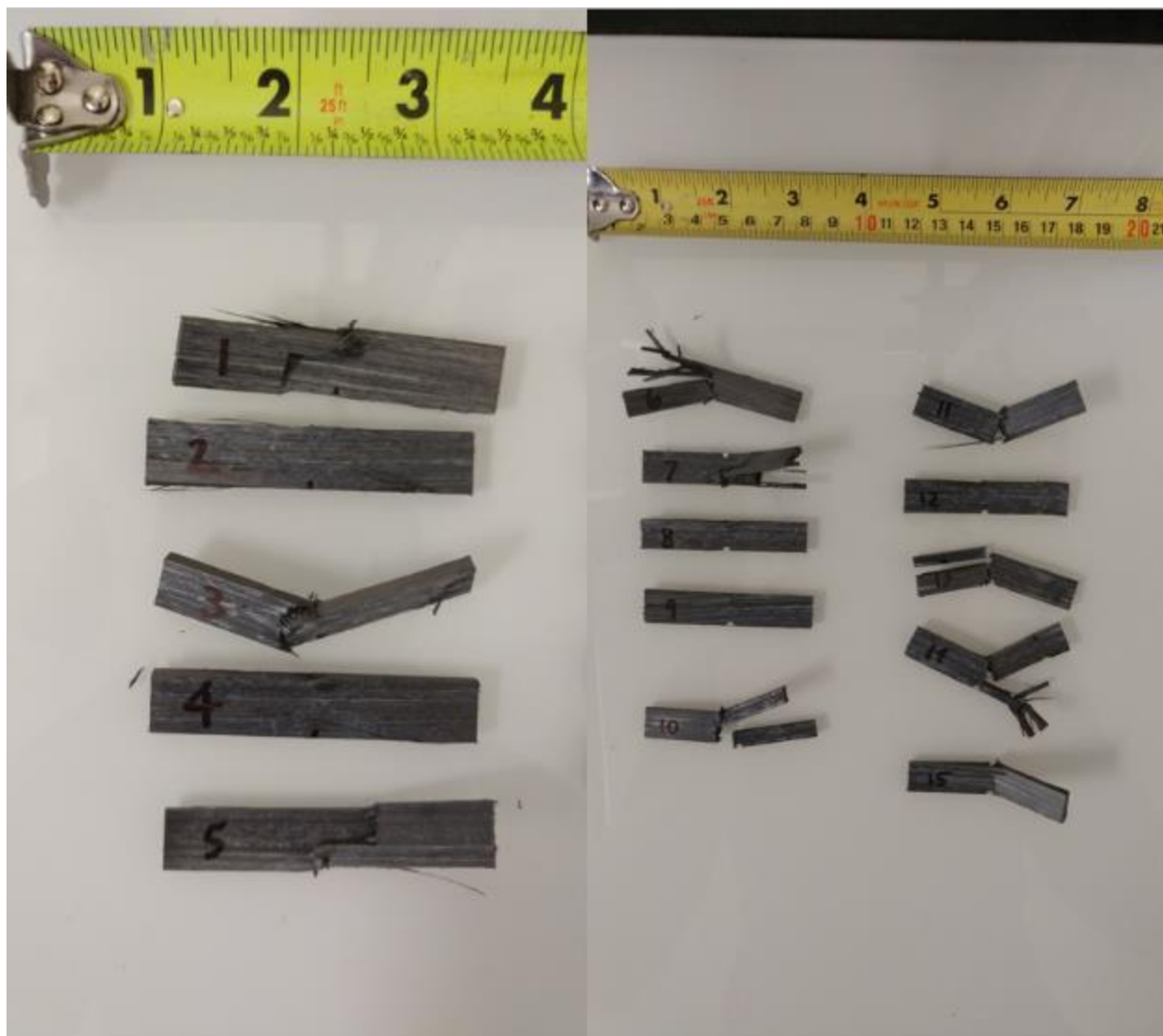
Figure 94 - Failures of unnotched 0-degree samples
