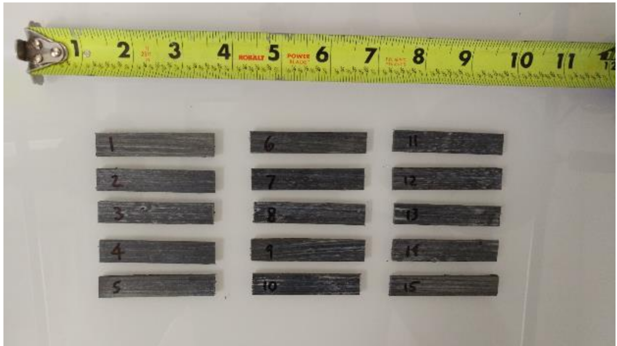
Figure 93 - Unnotched samples before testing
