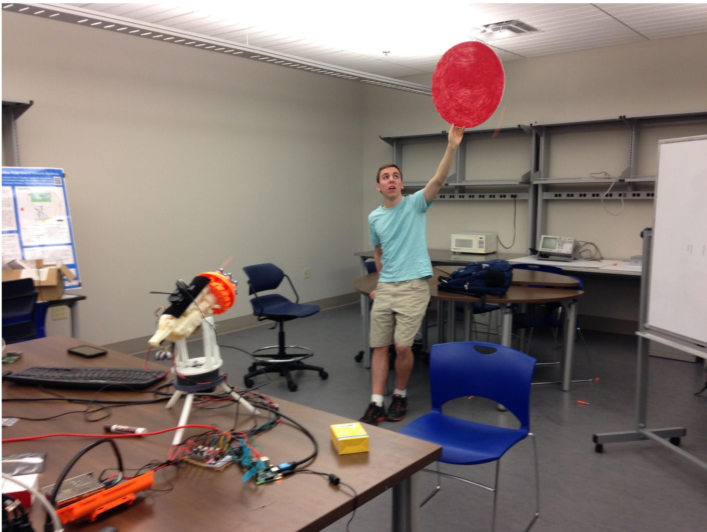
Figure: Kevin demonstrating the launcher’s tracking and firing capabilities A Nerf Swarmfire blaster has been mounted on a 3D-printed launching platform to form the main structure of the turret, with two Vex motors used to control the pitch and the yaw. A USB camera has been mounted on top of the gun.
