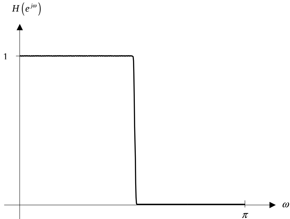
Figure 4.1. Frequency Response Magnitude of 495 th -Order Low-Pass Filter
