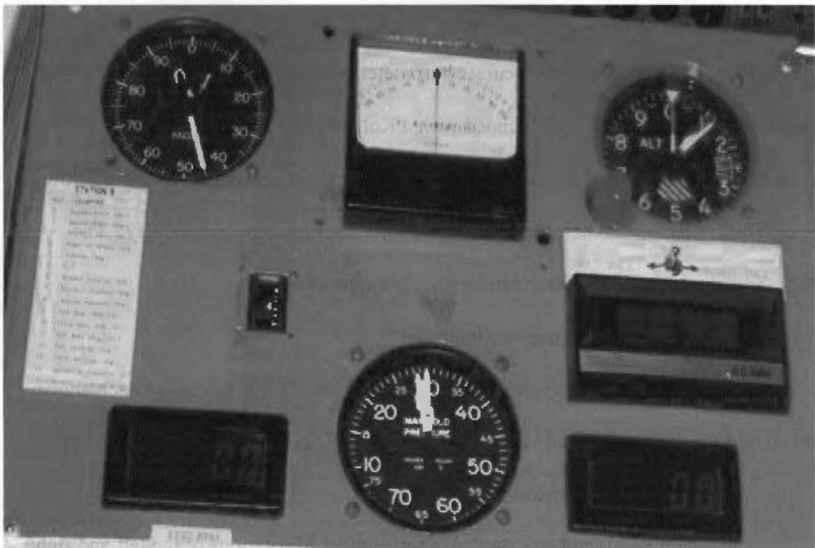
Figure 3.2 The Instrumentation Console Aboard the Piper Navajo
