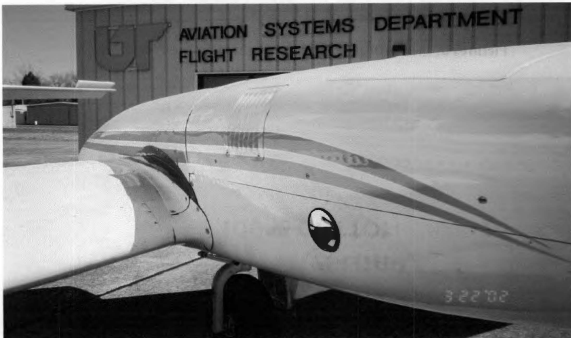
Figure C.3. Picture of the 75-Degree Left Inboard Nacelle Strake Mounted to the Left Engine Nacelle
