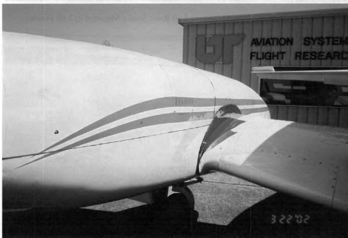
Figure C.3. Picture of the 75-Degree Left Inboard Nacelle Strake Mounted to the Left Engine Nacelle
