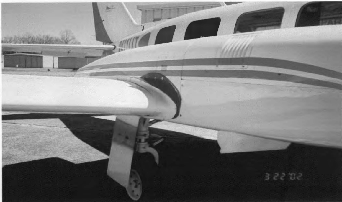
Figure C.5. Picture of the 75-Degree Left Outboard Nacelle Strake Mounted to the Left Engine Nacelle
