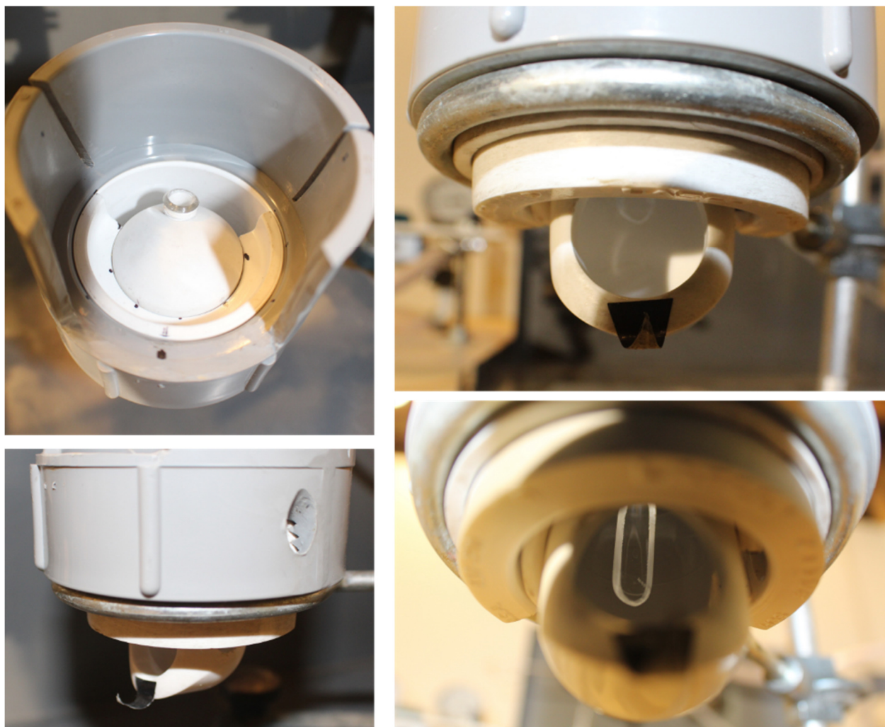
Figure 20: Exhaust channel and collections reservoir. Exhaust channel (upper left), collection reservoir (upper right), sample port and collection reservoir (lower left), and drip guide (lower right).
