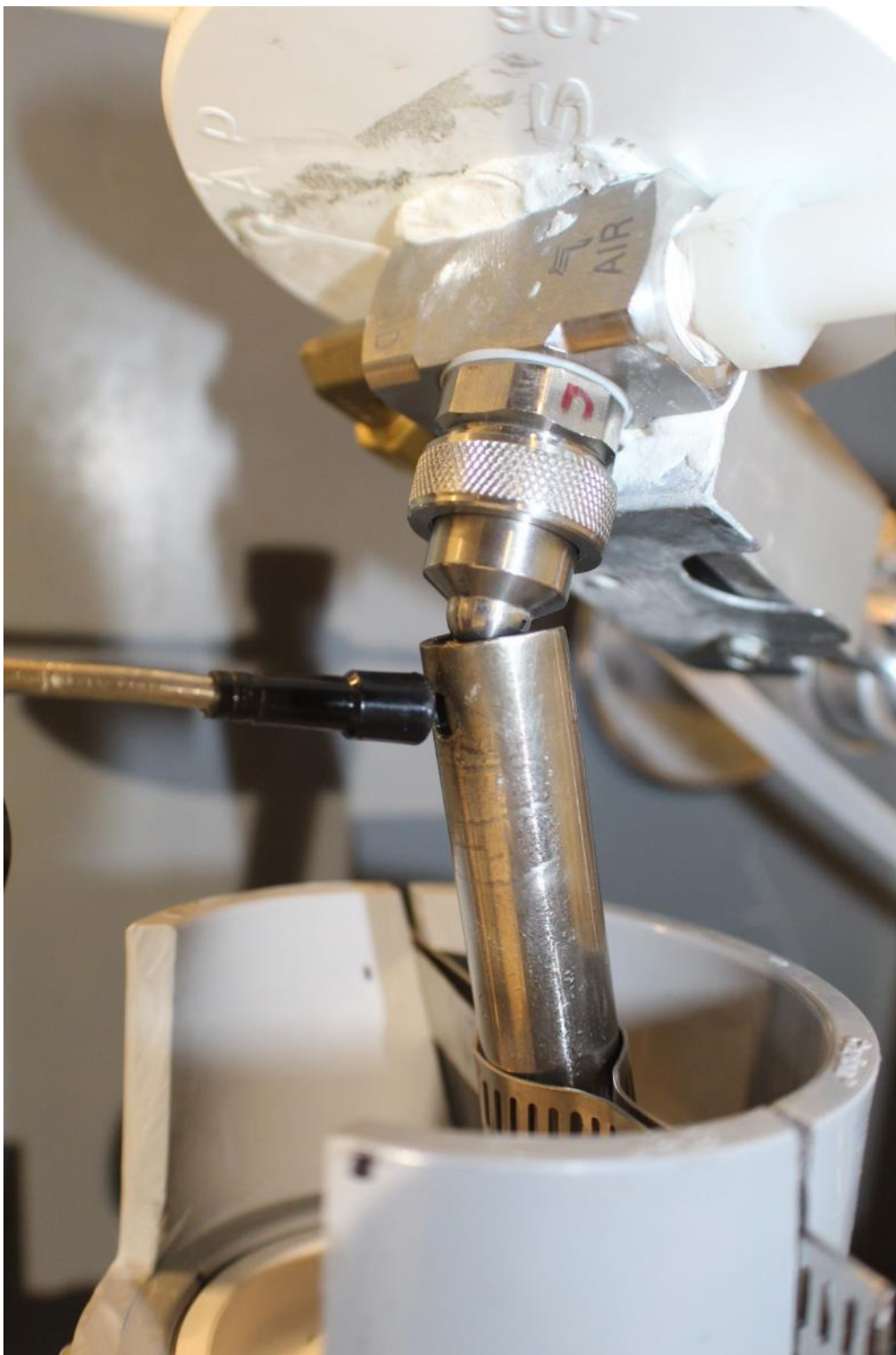
Figure 19: Relationship between REE injection nozzle, atomizer nozzle, and collection cylinder.
