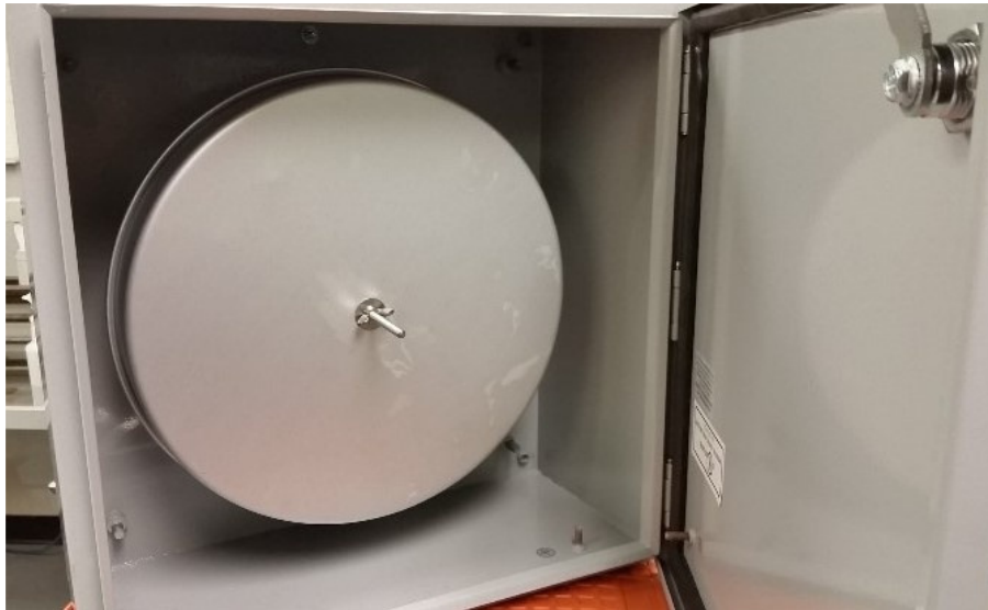
Figure 8: Rotary wheel apparatus used for aerosol deposition onto tape segments.
