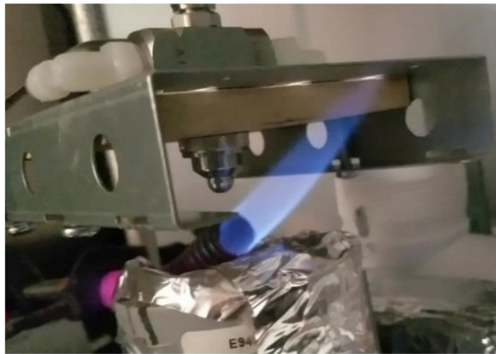
Figure 58: Thermal test of the PVC adapter and spray nozzle.
