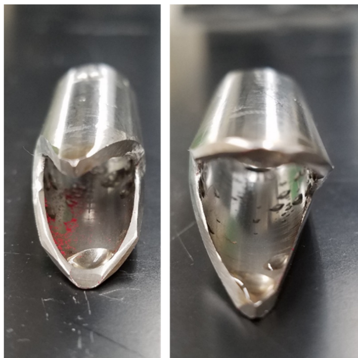
Figure 25: Powder paint deposits on the collection cylinder; back surface (left) and front surface (right).
