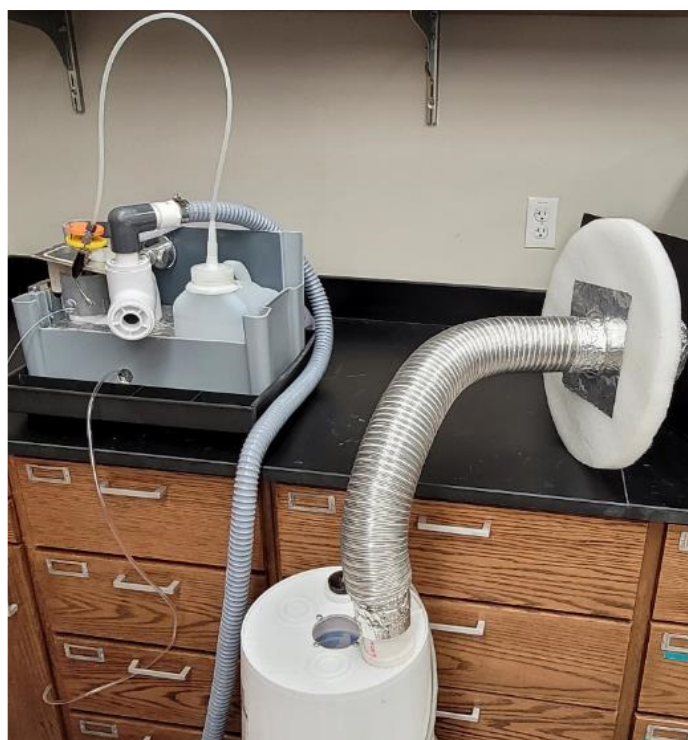
Figure 56: Adapted shop vacuum and snorkel exhaust.
