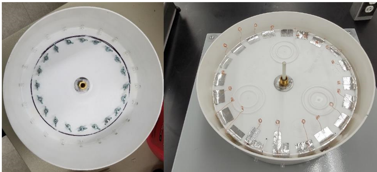
Figure 13: Wheel Apparatus Interior view (L) and Sample Collection Wheel (R).
