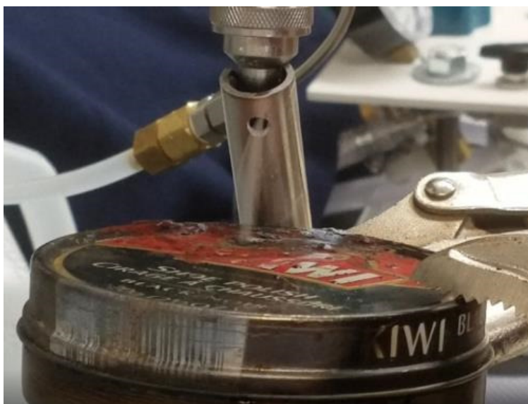
Figure 44: Buoyant smoke aerosols being drawn into the stainless-steel collection column via the low-pressure zone facilitated by the atomizer spray nozzle.
