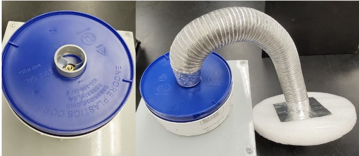
Figure 15: Exhaust Side of Wheel (L); Vacuum Adapter to the Snorkel Exhaust System (R).
