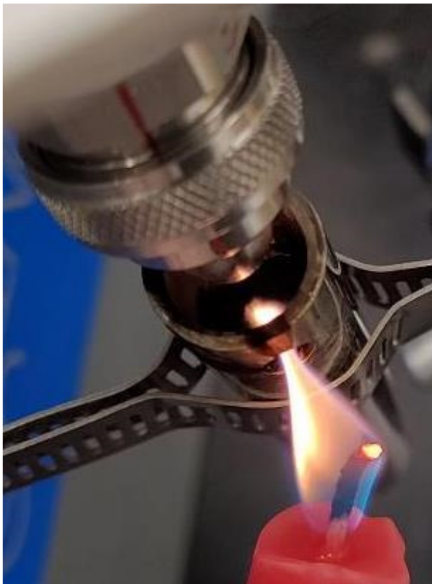
Figure 33: Flame test of the modified collection cylinder using compressed air at 25 psig and discharging into the ambient environment at 0 psig.
