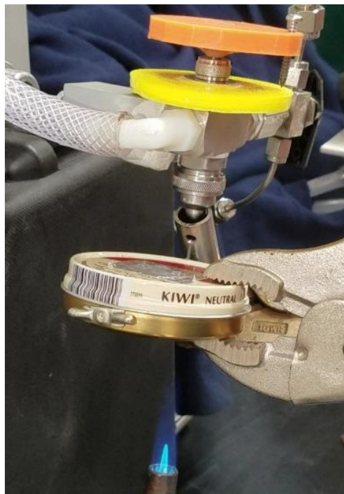
Figure 43: Special effects smoke being drawn into the stainless-steel collection tube. Note the column of smoke being expelled in the background.
