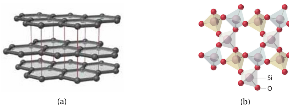
Figure 2.7: (a) Graphite covalent bond ( Chemistry 301, 2017 ). (b) Quartz covalent bond ( Averill and Eldredge, 2012 ).
