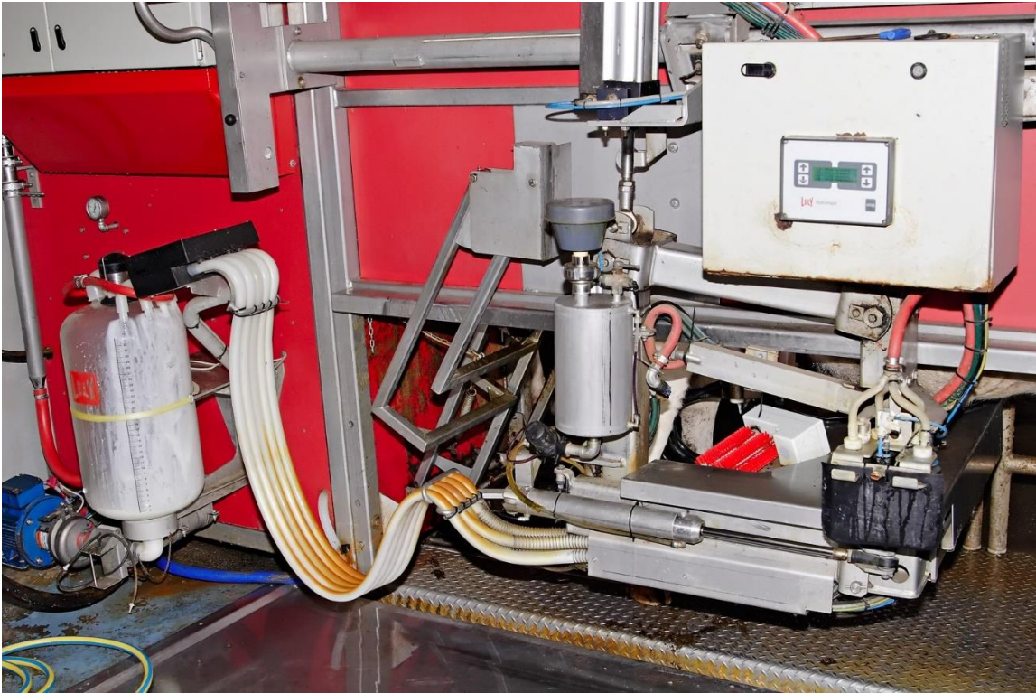
Figure 1.1. A 1995 automatic milking system at work (Lely, 2020).
