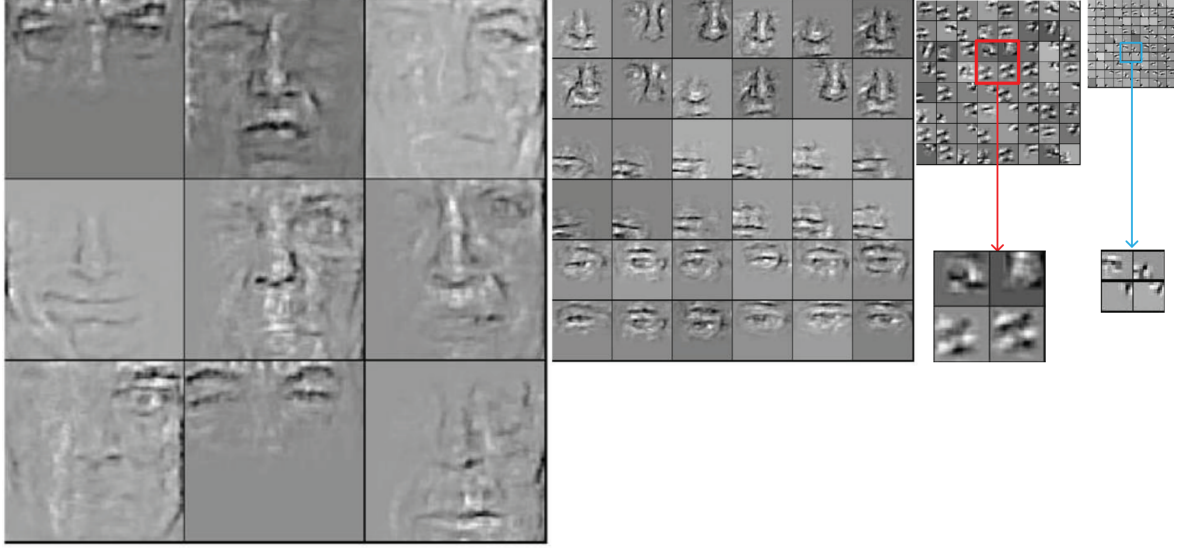
Figure 4.8: Hierarchical features learnt by the proposed ADN architecture. Feature generated by projecting the largest one activation from each layer back to the pixel space. From left, features learnt by layer 4 to layer 1. The activation from layer 4 has the receptive field covered the entire face. In the 3 rd layer, features are acquired at the facial parts level (nose, eyes, mouse, etc.). Features in 2 nd layer are mostly basic junction parts. In the 1 st layer, the primitive level Gabor-like features are learnt. The four-layer feature sets form the feature hierarchy. Noted that features are not in the original scale.
