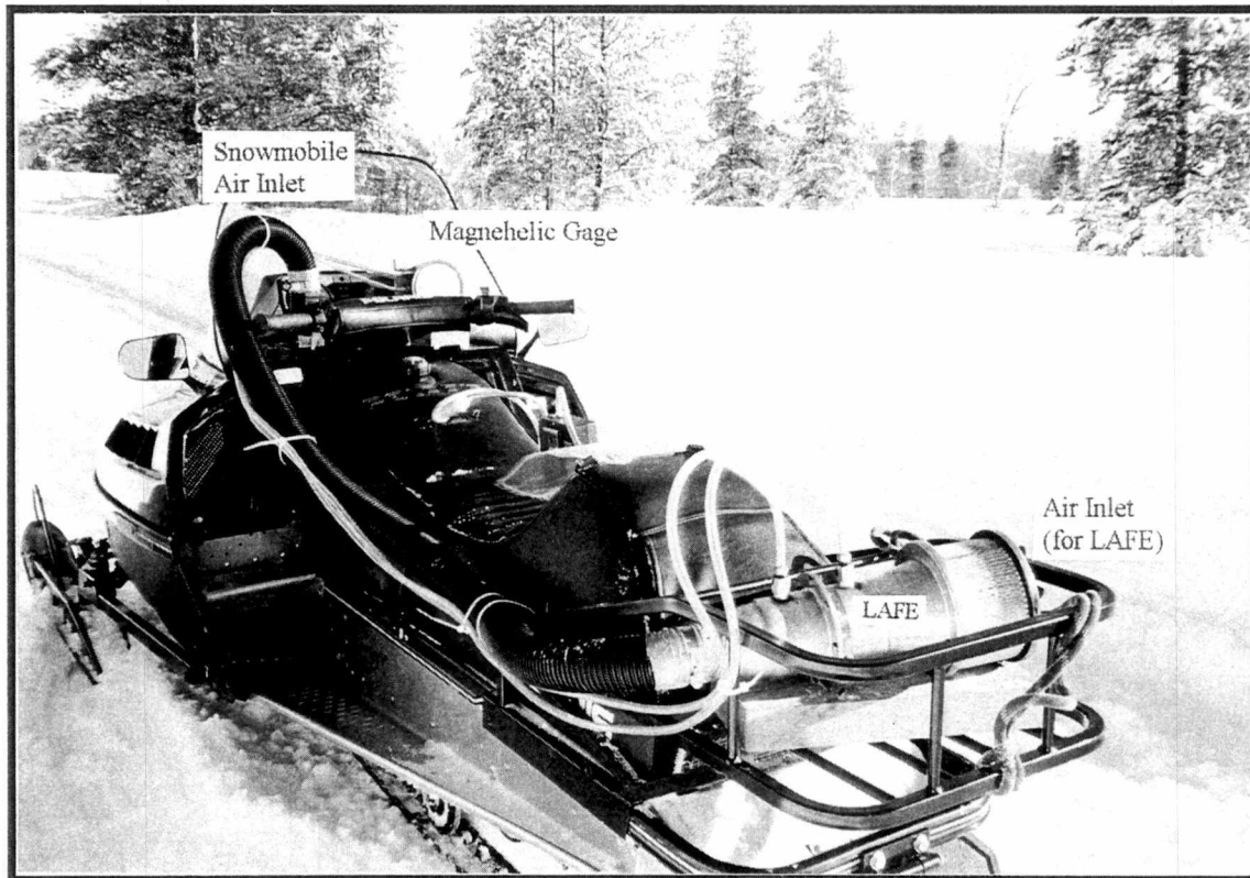
Figure 6 Picture of Exhaust Sampling Train
