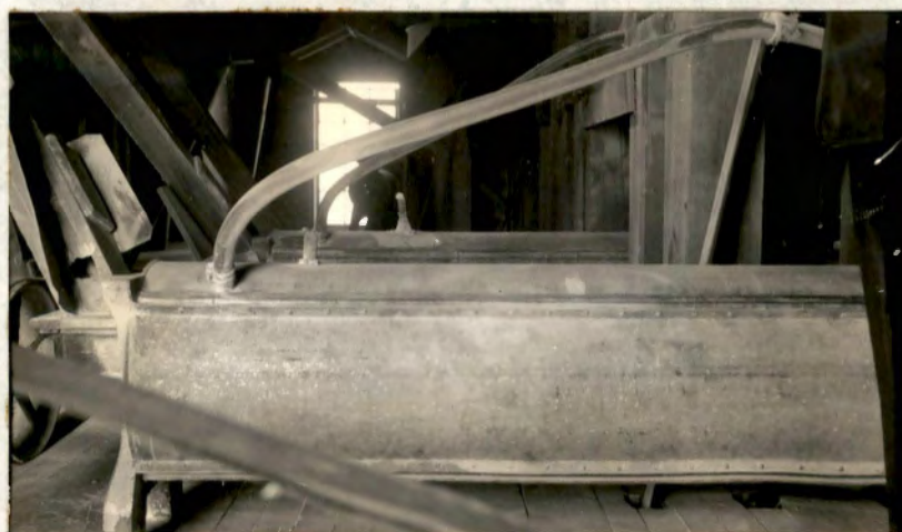
Figure 108. Batch mixer for adding self-rising ingredients to flour
