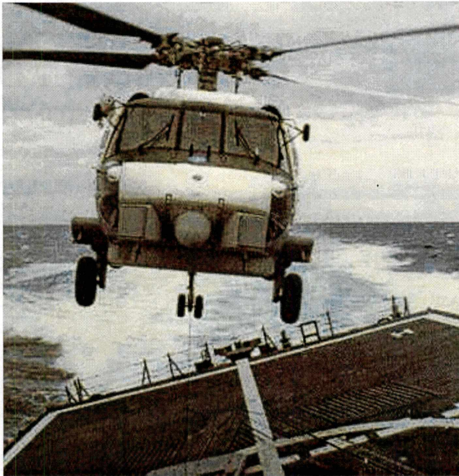
Figure A-5: HHRSD Hauldown Cable.
