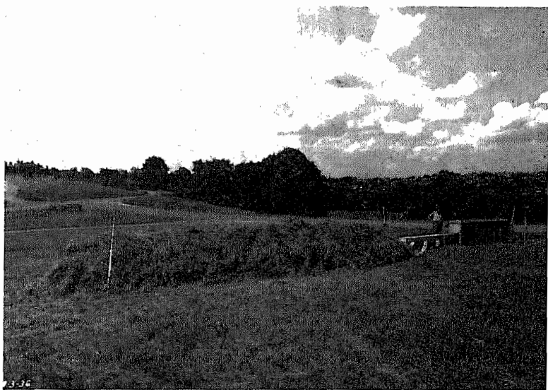
Fig. 2—Experimental method of drying hay in 30-foot ricks, 4 feet high and 5 feet wide. Air, tempered with heat, given off by a 3-h.p. engine, was liberated from 6-inch pipes under the hay.
