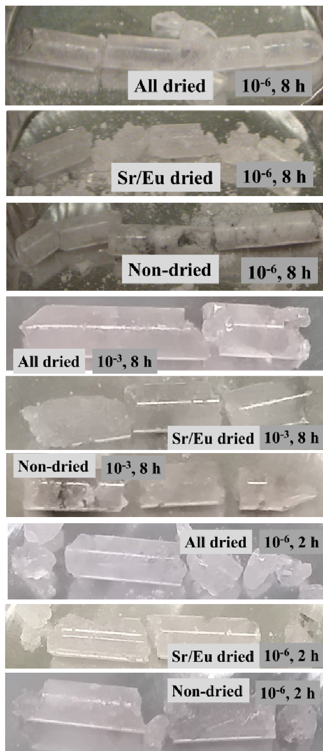
Figure 16. Samples of CsSrI 3 : 0.01% Eu after the third synthesis cycle.
