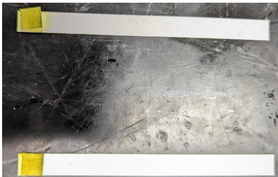
Figure 4.5: Photograph showing peroxide test strips after being dipped into the solution prior to irradiation (top) and after 10 minutes (bottom) during the photoediting of 4.1 under N_2 .
