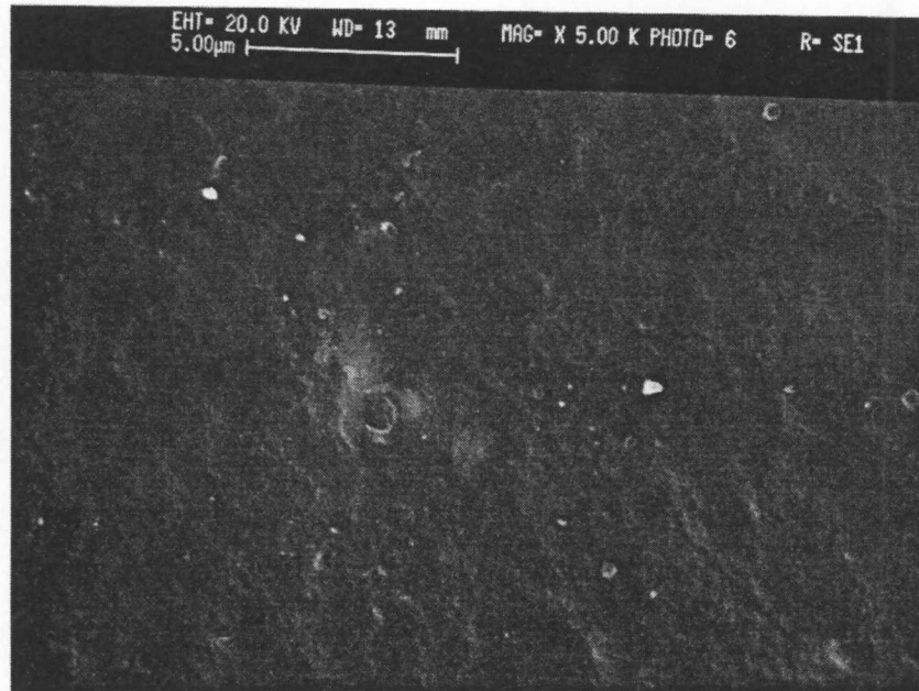
Figure 4.6 Scanning Electron Micrograph of (SEM) Untreated LDPE
