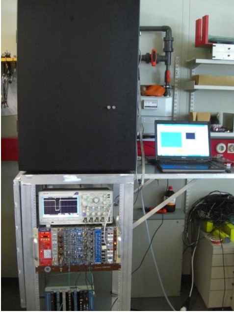
Figure 42: UT designed PMT testing Station consisting of a black box, oscilloscope, readout electronics and DAQ system.
