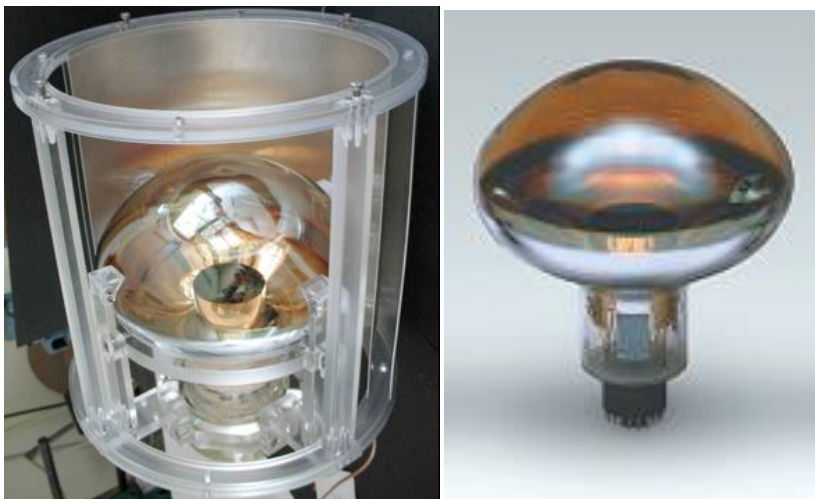
Figure 24: (Left) Hamamatsu R7801 PMT with acrylic mounting and Magnetic shield. A portion of the magnetic shield is removed to make the picture. (Right) Bare Detector PMT.
