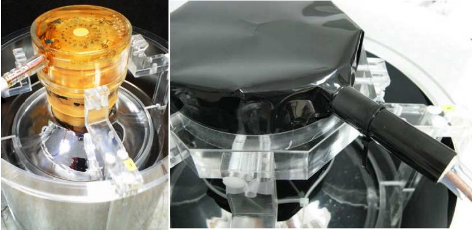
Figure 68: (Left) PMT base as it is in the Far detector. (Right) PMT base covered with black plastic to reduce light noise for the Near detector.
