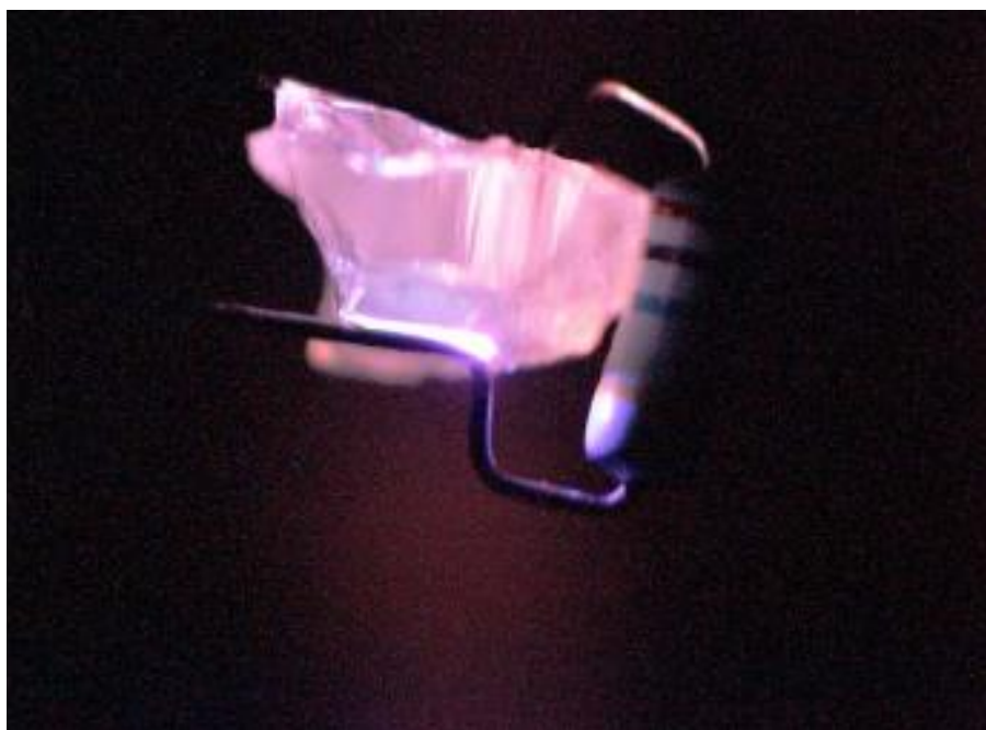
Figure 65: A sample of epoxy used in the PMT base is glowing when high voltage is applied.
