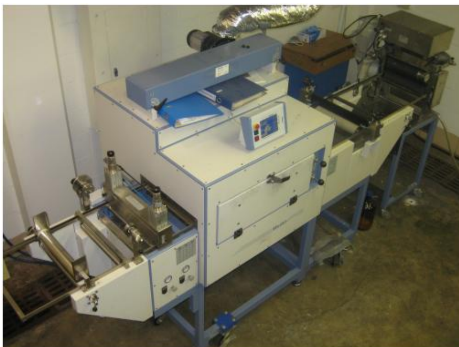
Figure 9 Mathis pad dry and cure equipment.
