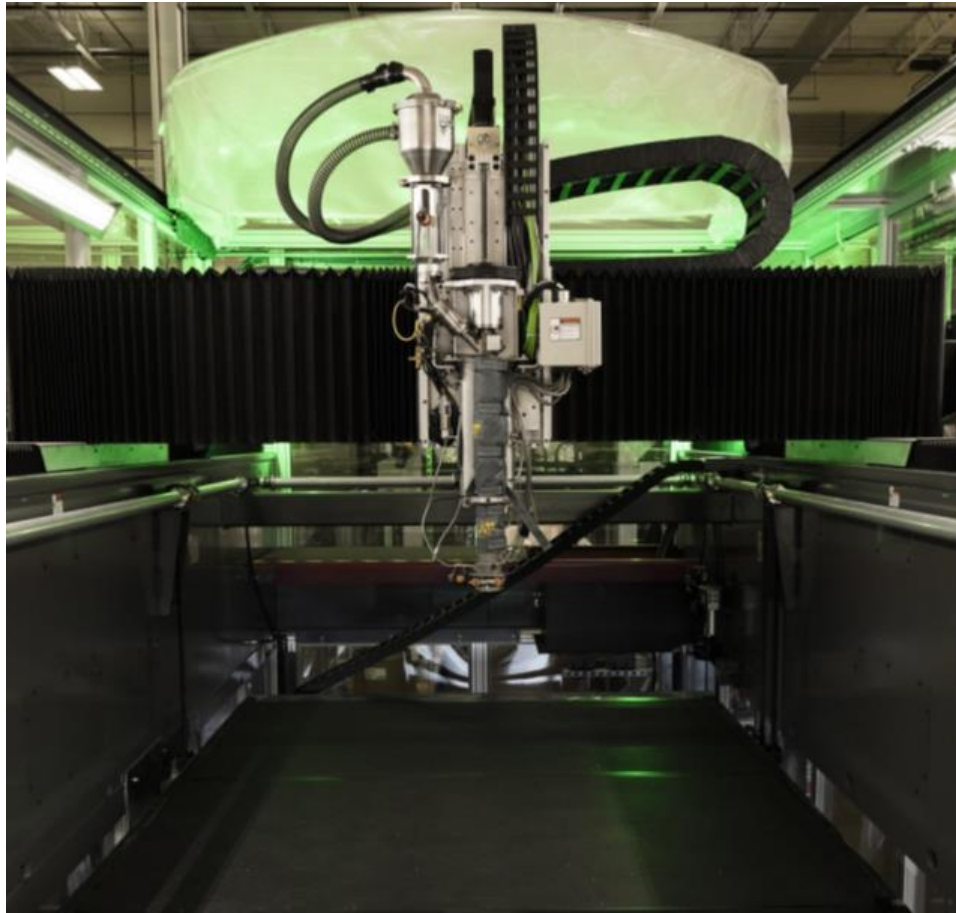
Figure 1.3 BAAM extruder set-up. Photo courtesy of Oak Ridge National Laboratory, US Dept. of Energy.
