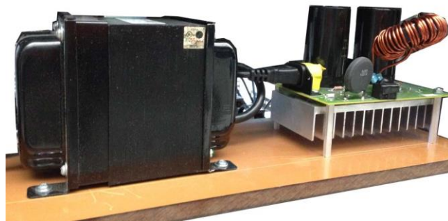
Figure 3-19 Photograph of half-bridge auxiliary power supply.
