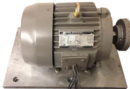
Figure 6-1 Photograph of three-phase 3 hp induction motor under test.
