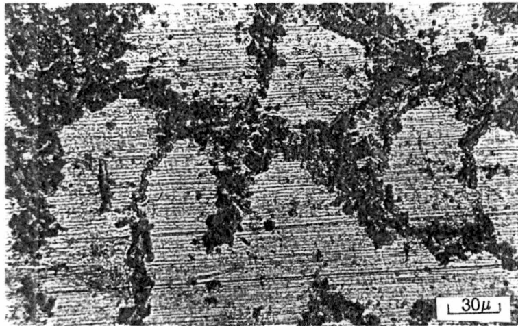
Figure 7. Microstructure of as-received A356 Al-10%SiC (p) MMC
