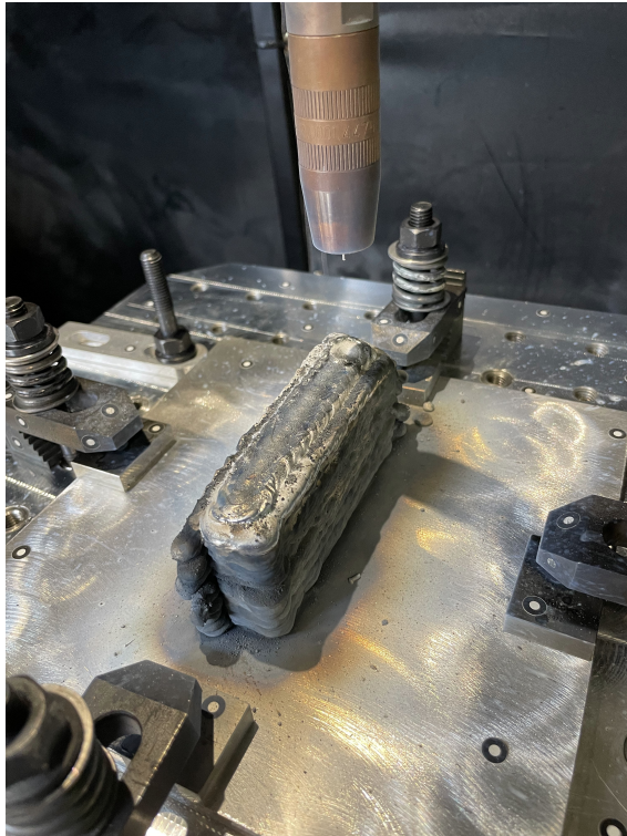
Figure 4.3: WAAM wall print several layers into the print.
