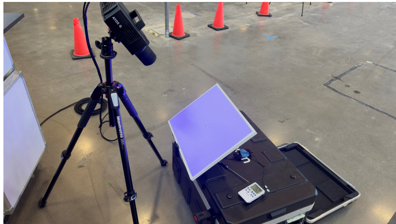
Figure 2.1: ATOS Q mounted to tripod for measurements.
