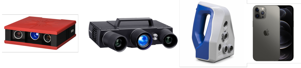
Figure 2.2: Optical CMSs studied in this work. From left to right: GOM ATOS Core 200, GOM ATOS Q, Artec Spyder, iPhone 15 Pro Max.
