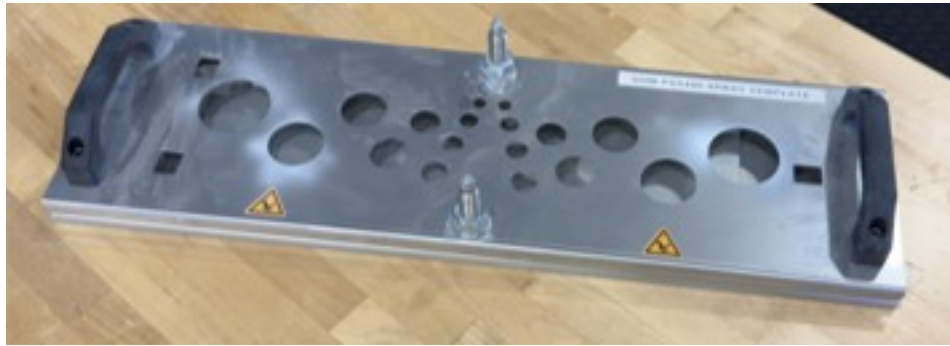
Figure 2.13: Cover for PSA400 artifact to enable spraying of spheres without coating scanner targets.
