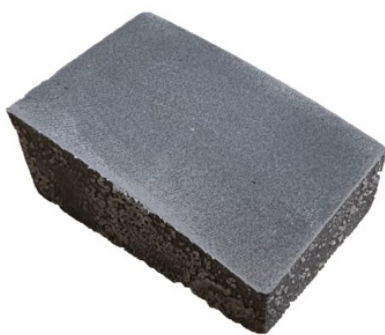
Figure B.7: Machined BJAM SiC sample.
