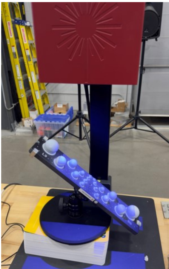
Figure 2.15: ATOS Core 200 mounted to lift with artifact mounted on rotary/tilt base.
