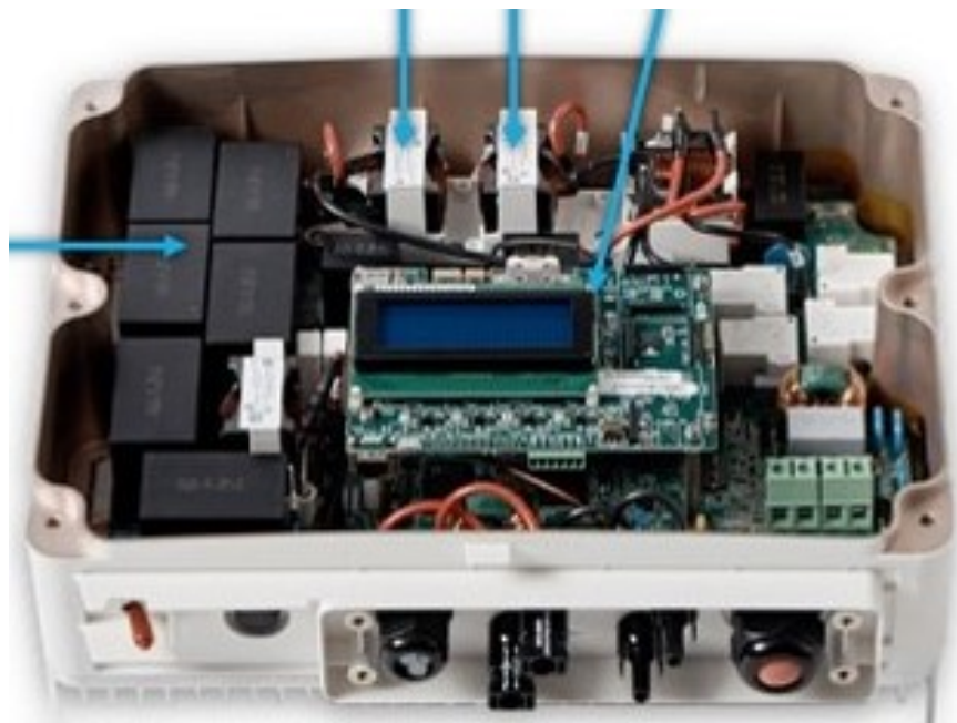
Figure 3.21: 7.6 kW SolarEdge HD Wave inverter [74].
