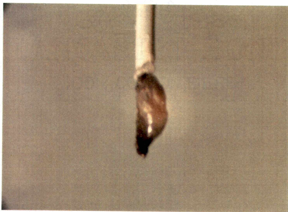
FIGURE 4.3 Typical Combustion Products at an Ambient pressure of 0.1 MPa (Low Pressure Regime).
