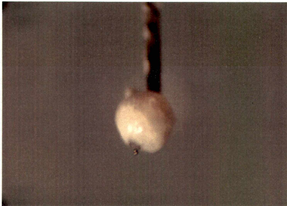
FIGURE 4.8 Typical Combustion Product at an Ambient Pressure of 0.8 MPa (Medium Pressure Regime)
