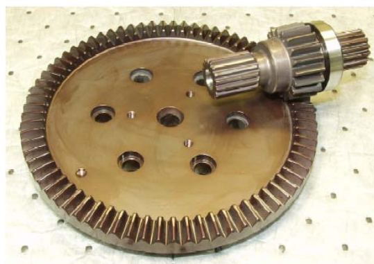
(b) A test face-gear drive in RDS-21 program [5].
