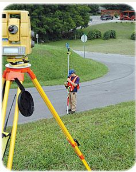
Glafenhein records data on the FC-2500 data collector as the prism receives signals from the GTS 800A robotic total station. Also mounted on the pole are an RC-2 infrared device (at top) and a Satel radio that provides a communication link back to the total station. Photo by Robert Freeland
